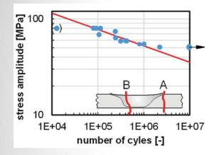
Comparing the Wöhler curves, it shows the excellent fatigue strength of a friction stir welding connection relating to base material EN AW 6016 T4.
