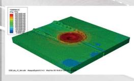
Calculated temperature fields for friction stir welding (above) and resistance spot welding (below)
