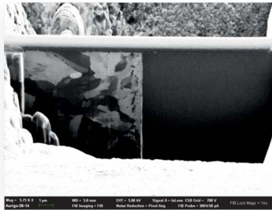
FIB preparation of a dissimilar weld (high temperature steel and nickel base alloy)
