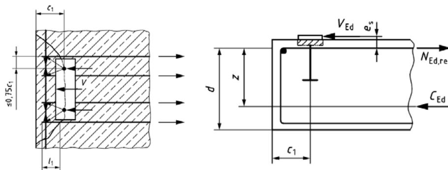
Fig. 1: Strut and tie model for suppl. Reinf. under shear loading according to EN 1992-4 [1]
