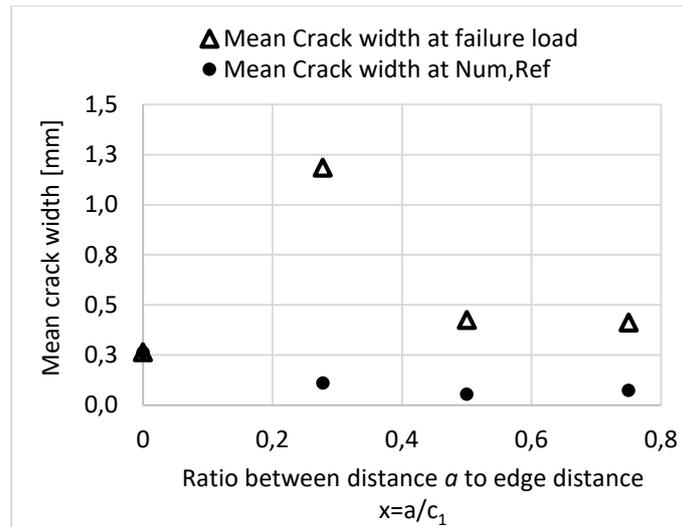
Fig.7: Mean crack width as a function of the ratio between  $a/c_1$
