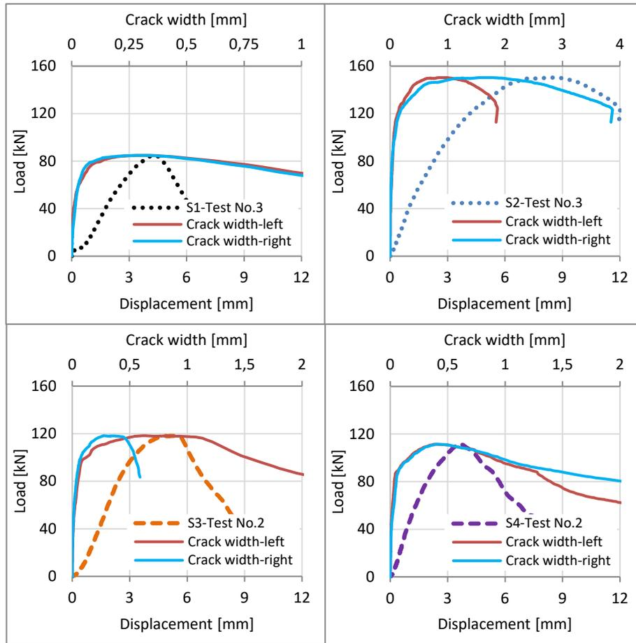
Fig. 6: Load displacement and crack width curves obtained from the shear tests on single anchor without and with post-inst. reinforcement
