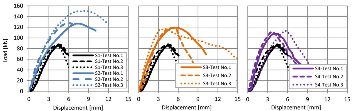
Fig. 4: Load-displacement curves for different Series: S1-Reference (black), S2-with 2 x d10;  $a = 50$  mm (blue), S3-with 2 x d10;  $a = 90$  mm (orange) and S4-with 2 x d10;  $a = 135$  mm (purple)
