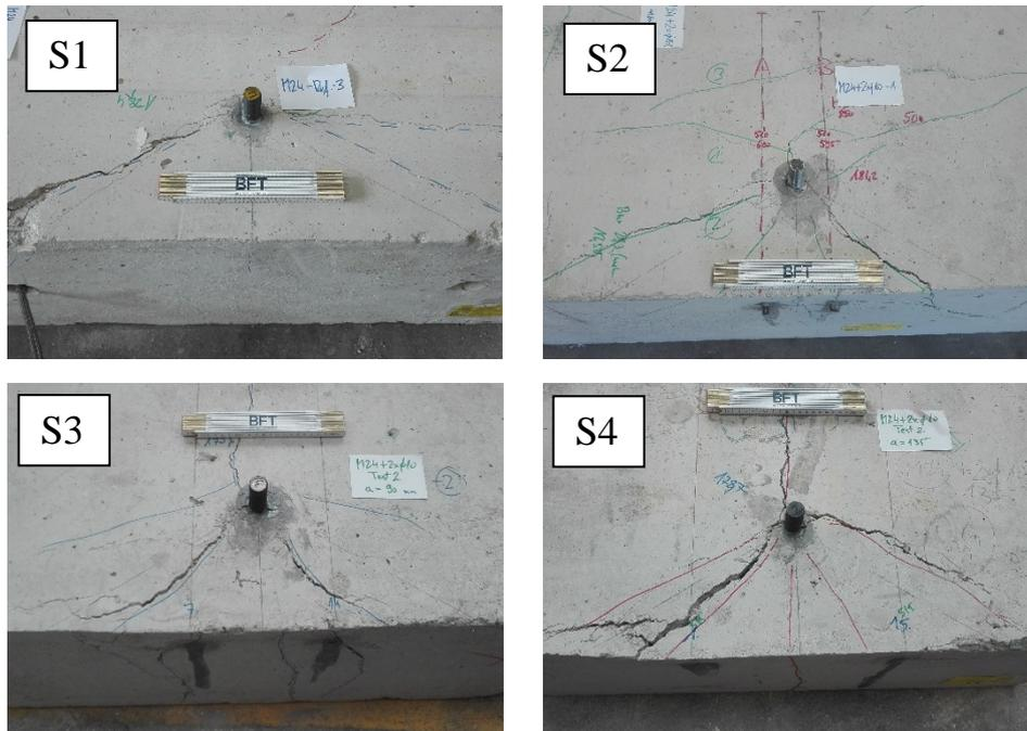
*Fig. 5: Typical failure mode obtained from the shear tests on single anchor without and with post-inst. rebars*
