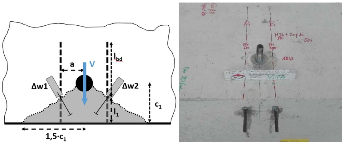
Fig. 2: Schematic (left) picture (right) from the installed bonded anchor with post-installed supplementary reinforcement as a strengthening under shear loading
