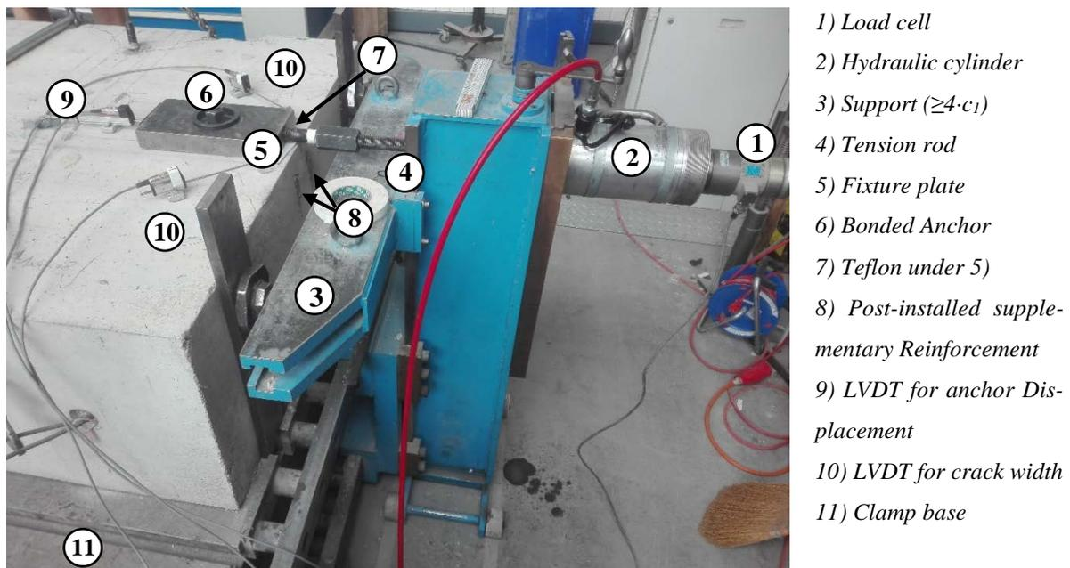
Fig. 3: Test setup for shear loading for single anchors with details
