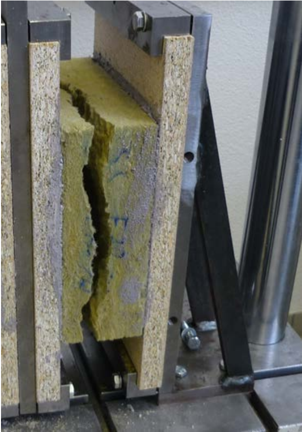
Fig. 4: Specimen from stone fibres after failure
