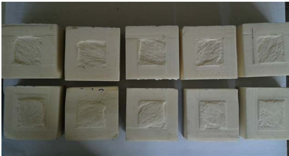
Fig. 2: Test specimens of XPS after the tensile strength test (cohesion break)
