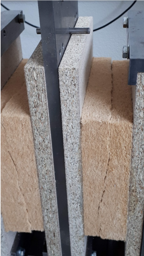
Fig. 3: Specimen from wood fibres after failure
