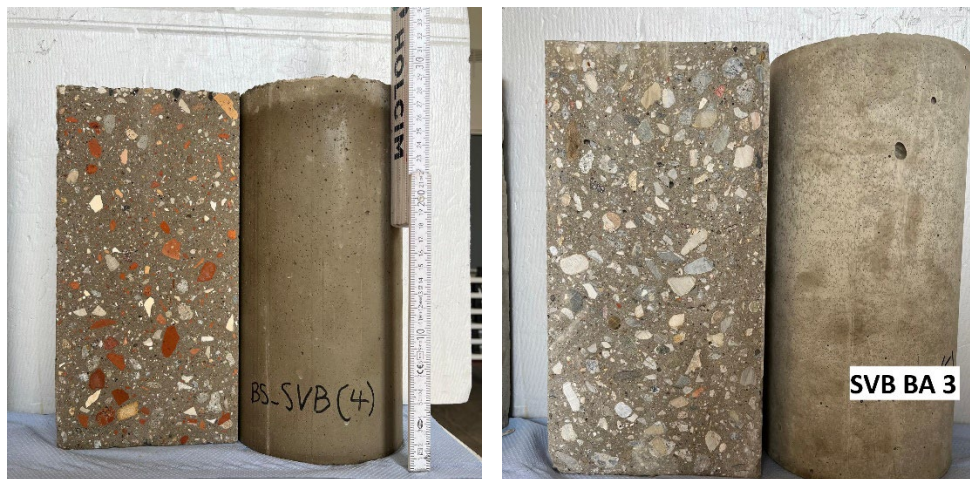
Fig. 3: Sedimentation tendency in the cylinder of mix BS 4 (Type 2) and BA 3 (Type 1) [1]
