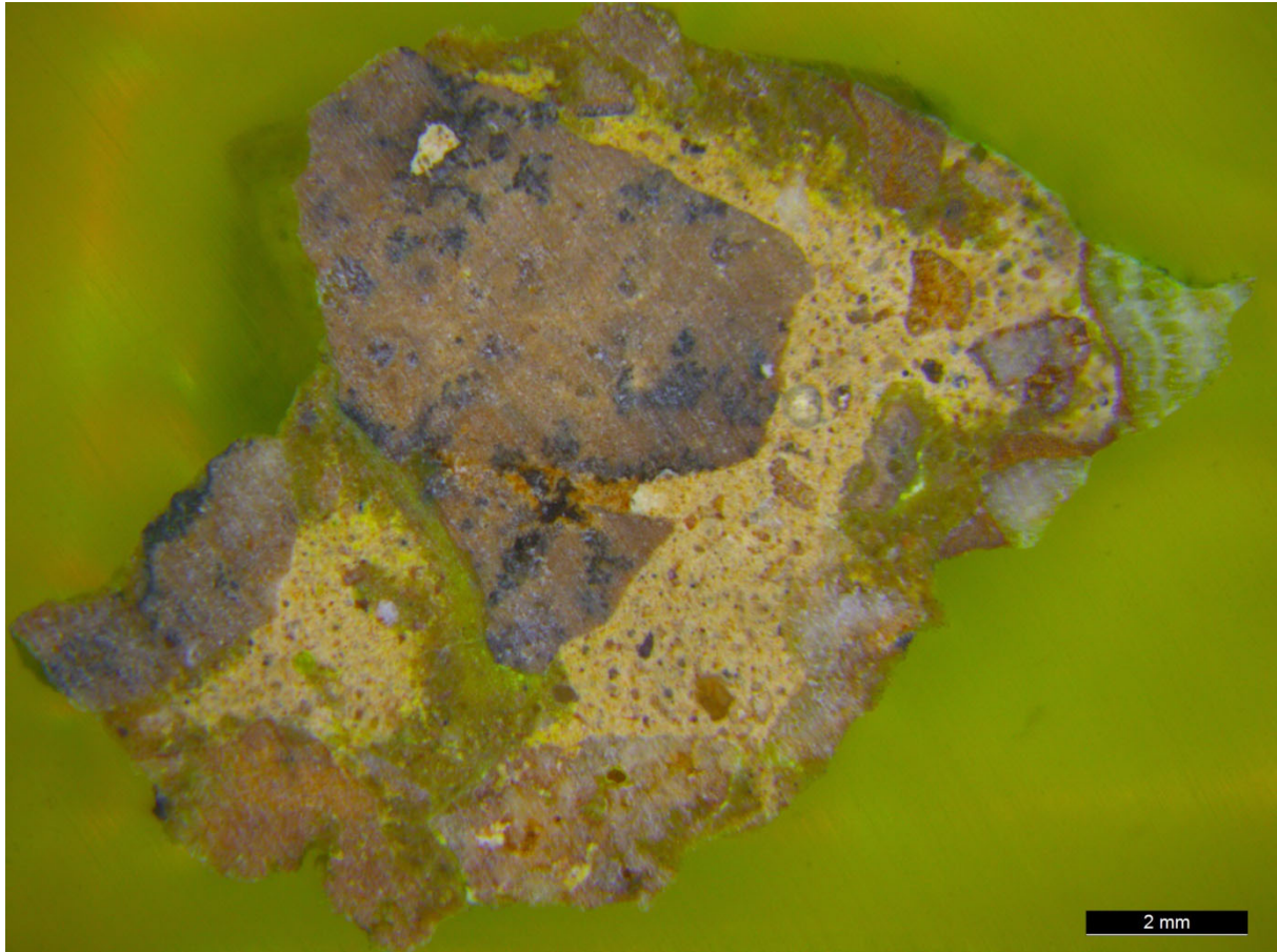
Fig. 4: Overview of the thick section from the “concrete” sample, embedded in fluorescent epoxy resin. The binding material appears bright, with only small particles inside. There is one large aggregate in the center and more remnants of other aggregates along the sides.
