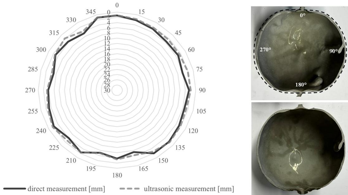
Fig. 4: Obtained measurements and radial visualization scaled by 2.5 (left), cut-open view (right) of the mineral hollow body no. 22.02.-2 in the same plane (axis A)
