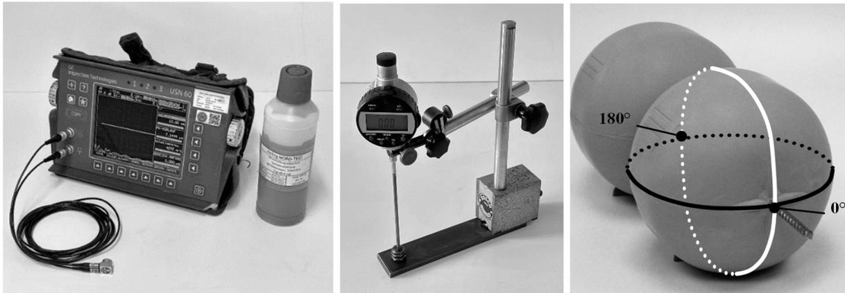
Fig. 3: Ultrasonic testing device (left), dial gauge (middle) and respective measuring axes A (black) and B (white) (right)
