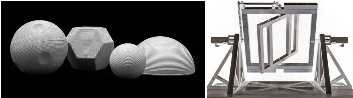
*Fig. 1: Different mineral hollow body geometries (left) and prototypical biaxial centrifuge for their production (right) [8]*
