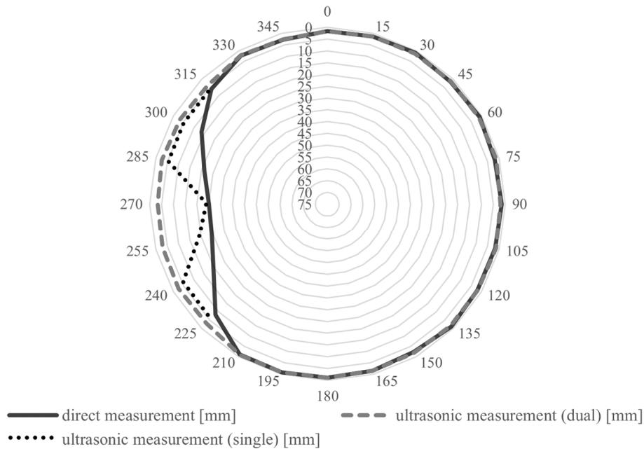
*Fig. 7: Resulting measurements of dual-and single-element transducers in radial unscaled visualizations of the mineral hollow body no. 28.02-3 in the orthogonal plane (axis B)*
