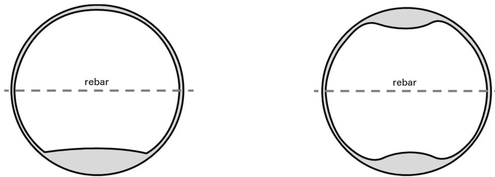
Fig. 2: Cross-sectional view of two critical material distribution patterns: sinking to bottom after rotational moulding process (left) and ring-shaped accumulation (right)
