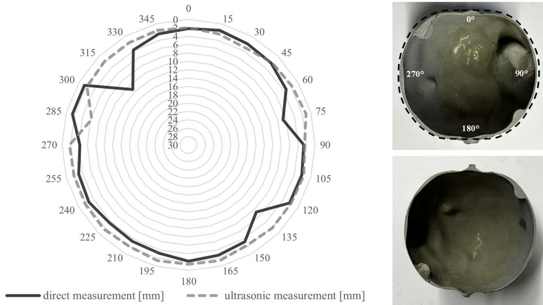
*Fig. 5: Obtained measurements and radial visualization scaled by 2.5 (left), cut-open view (right) of the mineral hollow body no. 22.02-3 in the same plane (axis A)*
