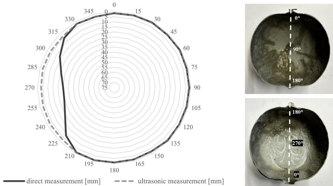
Fig. 6: Obtained measurements and radial unscaled visualization (left), cut-open view (right) of the mineral hollow body no. 28.02-3 in the orthogonal plane (axis B)
