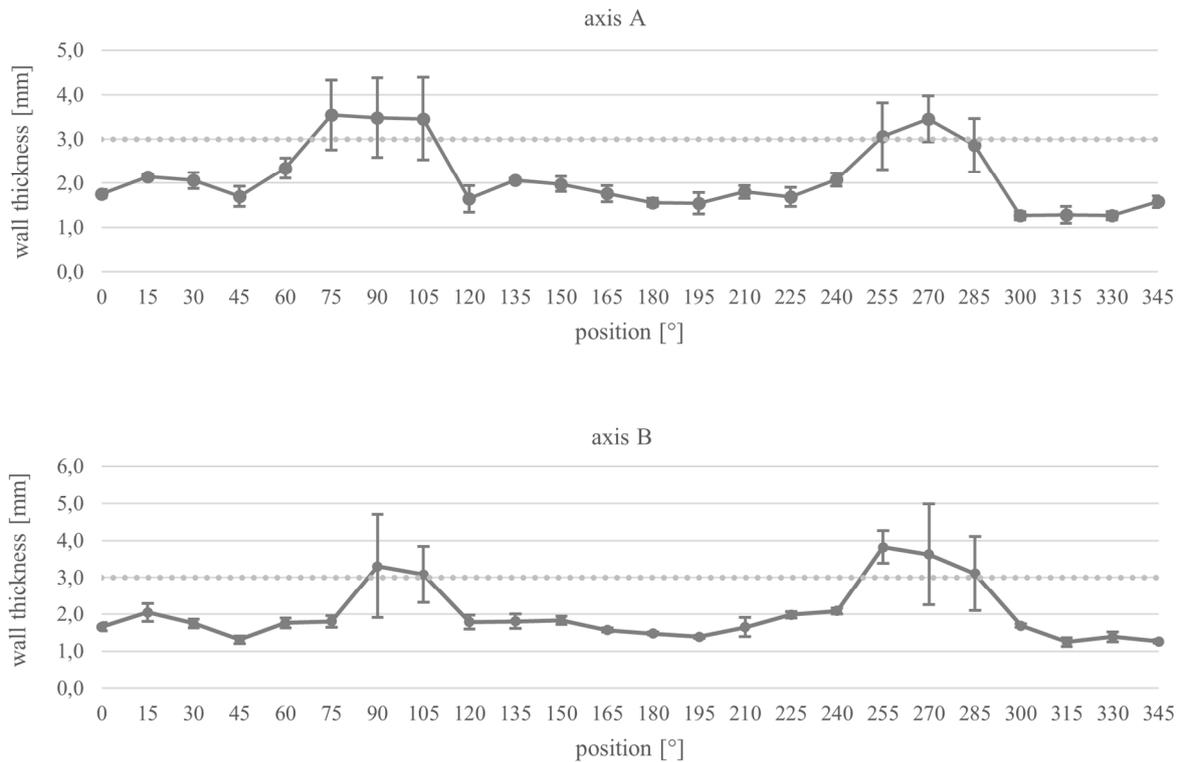
Fig. 8: Resulting ultrasonic measurements and linear visualizations of sample specimen from past production cycles
