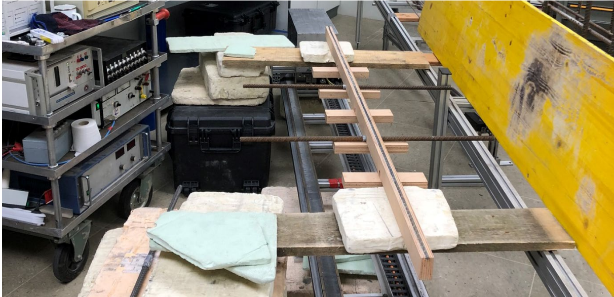
Fig. 14: Experimental setup- fractured prestressing steel with varying positions and combinations of rebars
