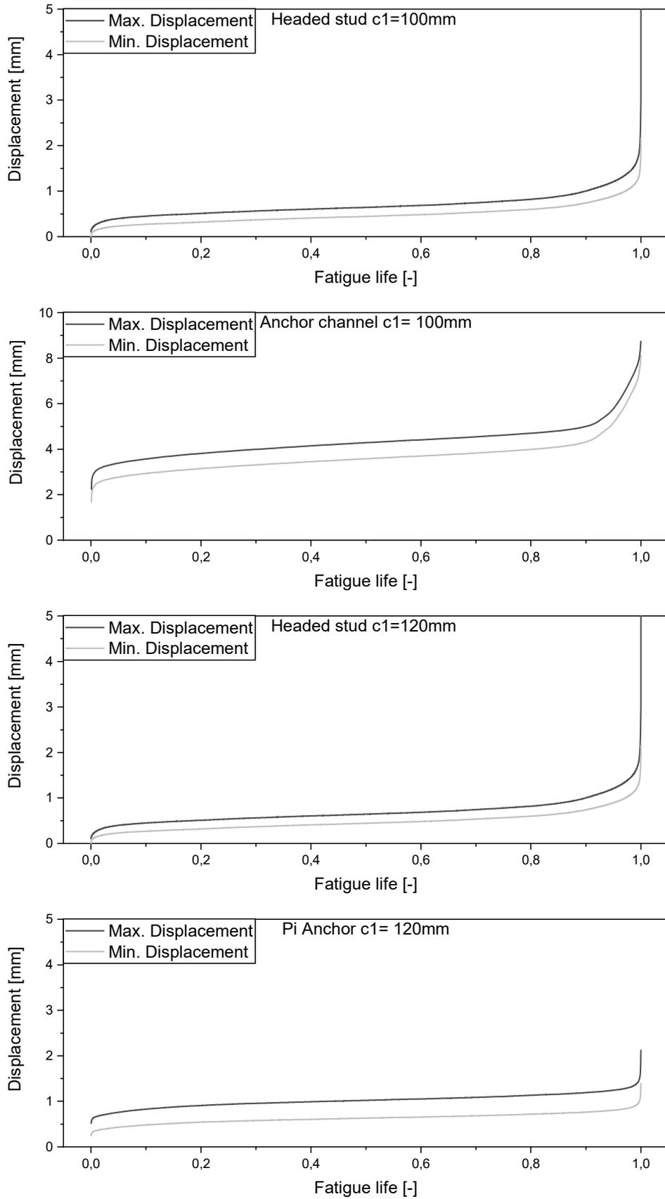
Fig. 6: Displacements of the fatigue tests at a load range of 65% of the ultimate load
