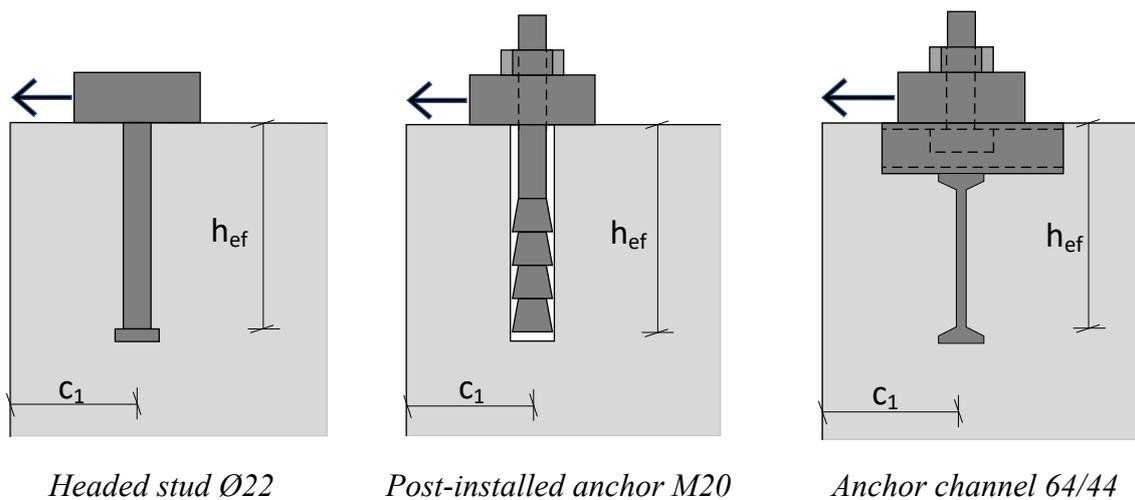
*Fig. 1: Graphic of tested fasteners located close to the edge*
