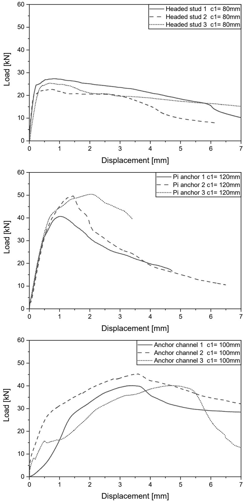
Fig. 3: Load-displacement curve of the static tests
