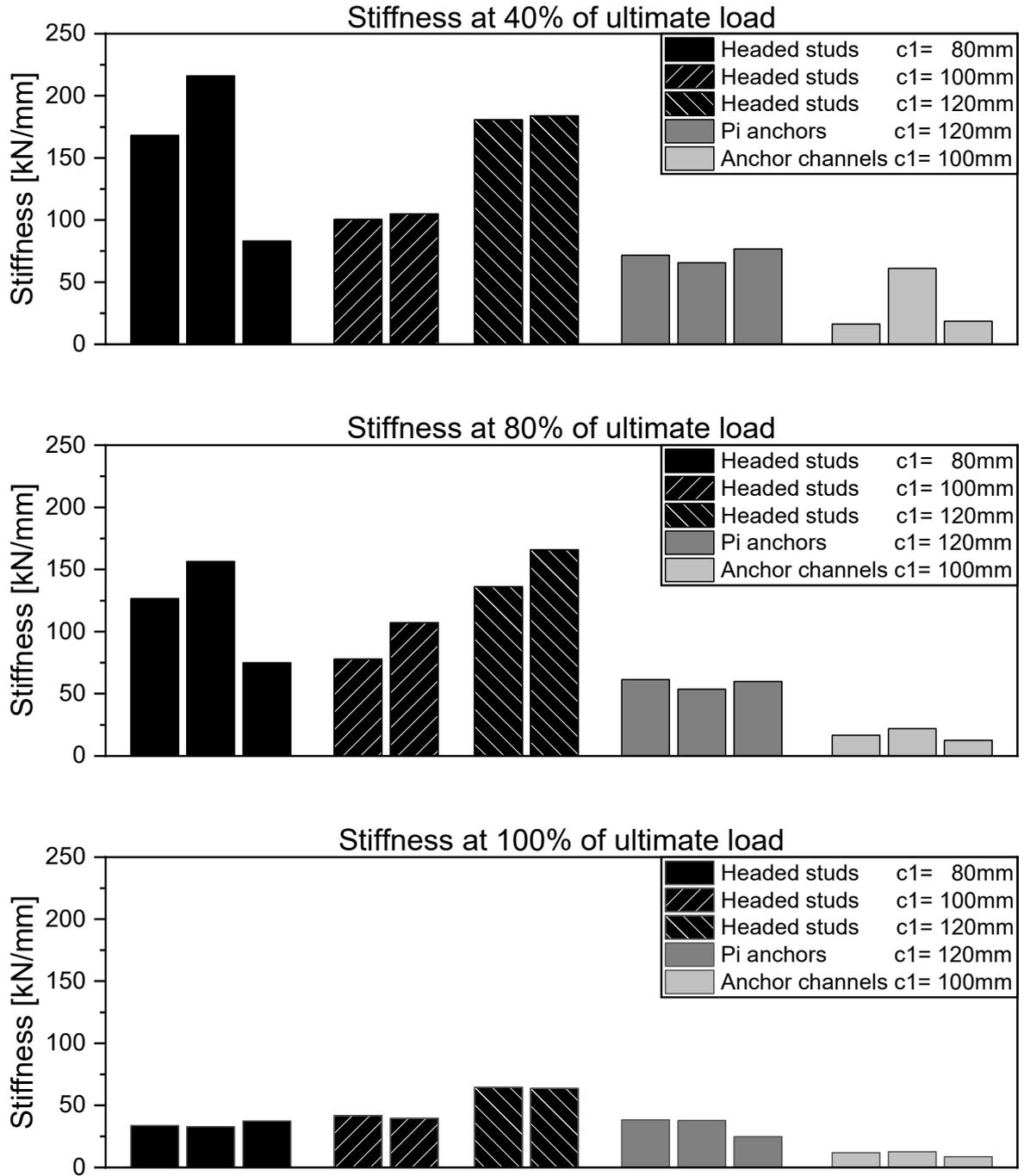
Fig. 4: Stiffness of the individual static test series at 40%, 80% and 100% of the ultimate load
