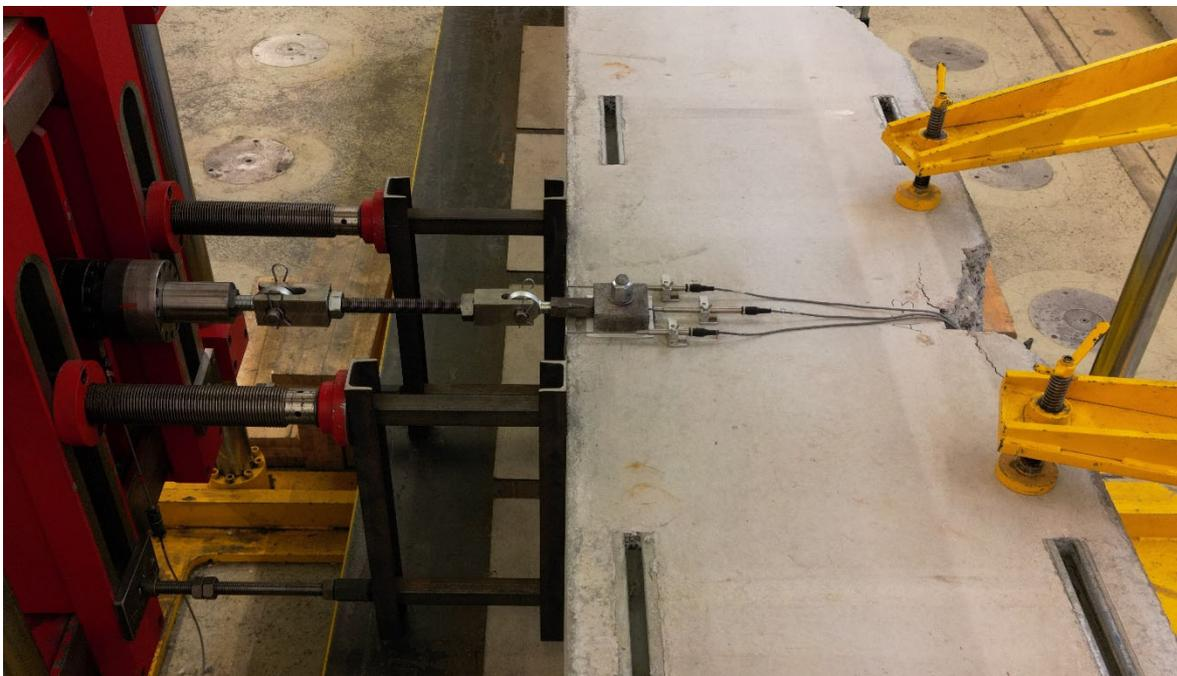
*Fig. 2: Test set-up and measuring equipment of the shear load tests*
