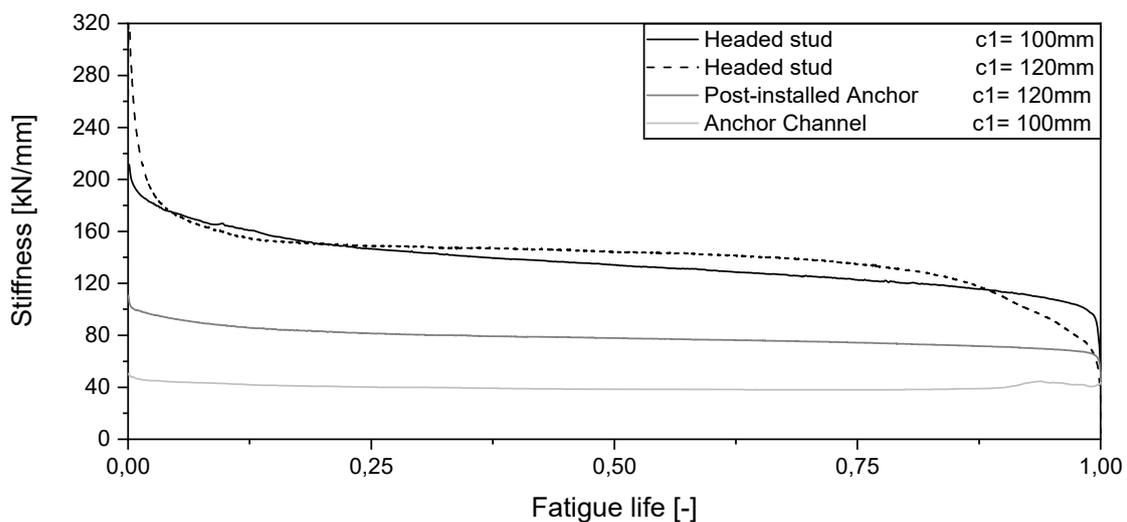
Fig. 7: Course of the stiffness over the fatigue life of the individual fasteners
