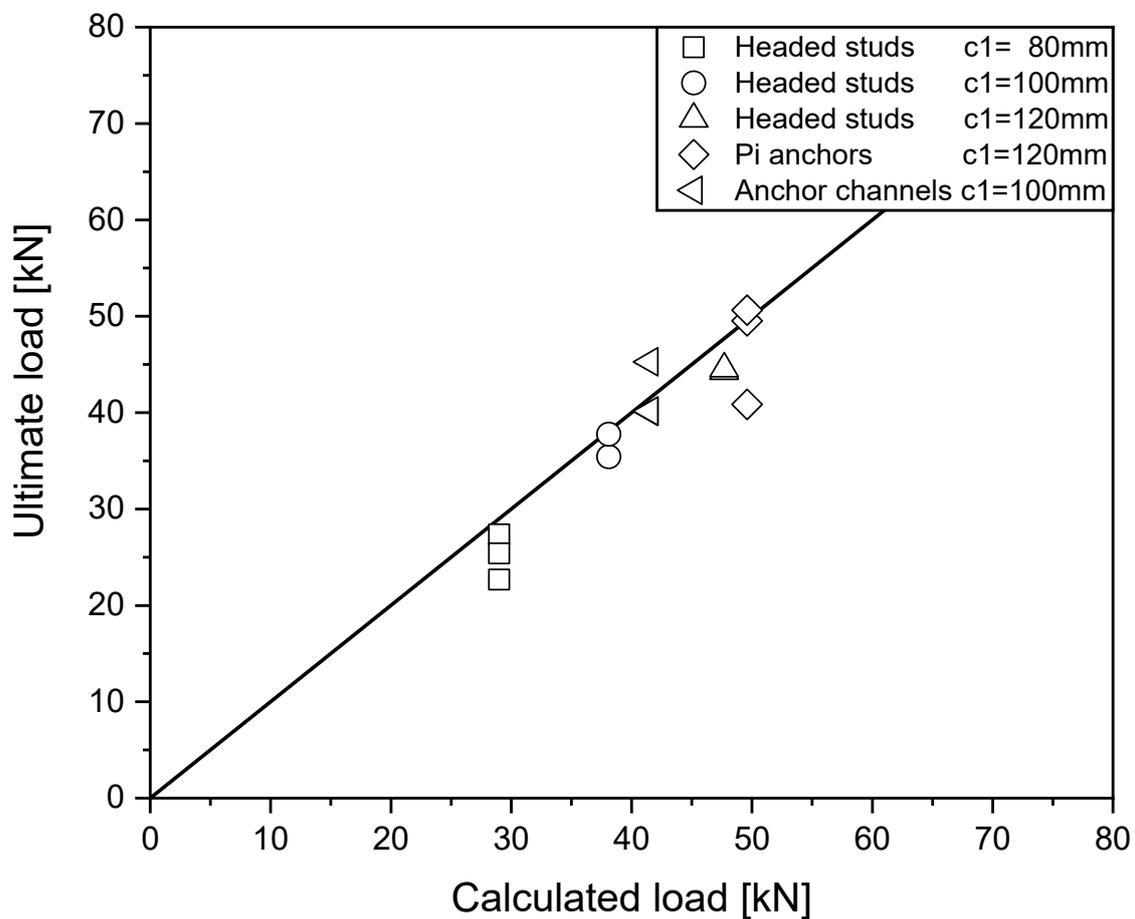
Fig. 5: Ultimate test loads compared with calculated average loads
