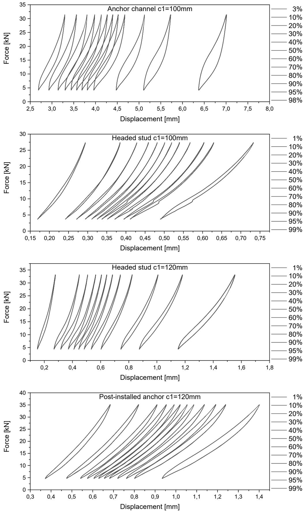
Fig. 7: Hysteresis of the fatigue tests at a load range of 65% of the ultimate load
