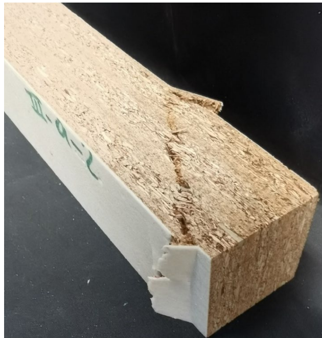
Fig. 12: Particle board compression strength specimen with typical failure
