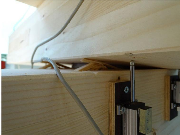
*Fig. 19: Typical failure appearance in the bending tests (here specimen 1b-01); the pull-out of the screws between diagonal and bottom chord*
