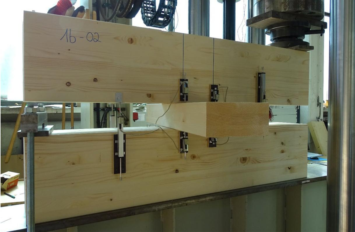
Fig. 11: View of realized test setup for determination of  $K_{My}$  stiffness (= bending about the y-axis)
