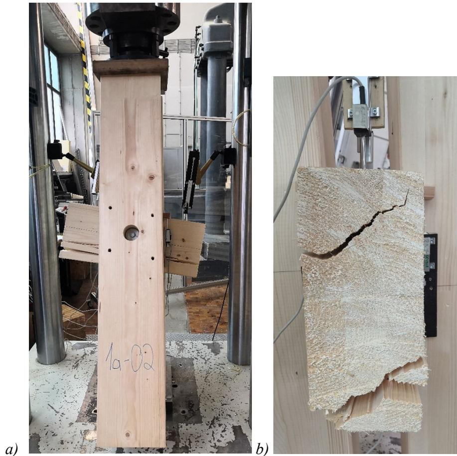
Fig. 13: Typical fracture appearance (here specimen 1a-02) with crack formation in the diagonal
