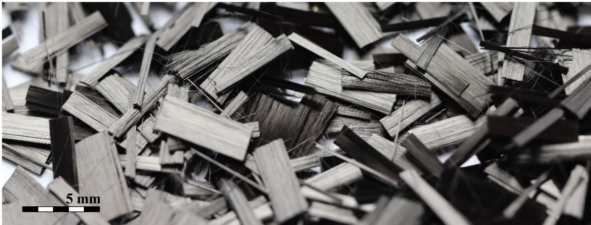
Fig. 3: Close-up of carbon fibre bundle
