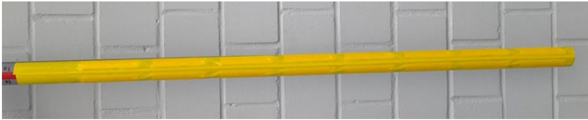
Fig 3: Probe with insulation covering the entire surface of the electrodes
