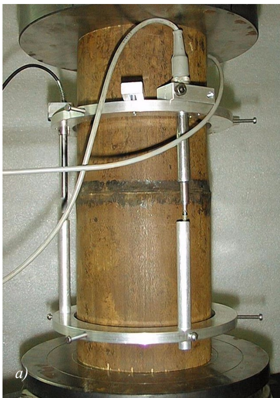
Fig. 3: Pictures of the realized compression test set-ups a) for a ZERI specimen of type B2, b) for a DIHAD specimen with D = 100 mm
