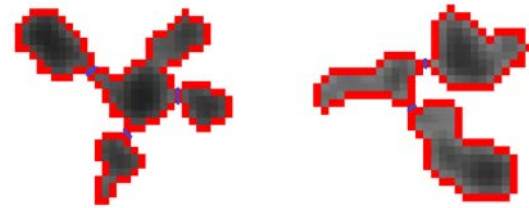
Fig. 5: Exemplary representation of particles erroneously combined from several individual particles by the software
