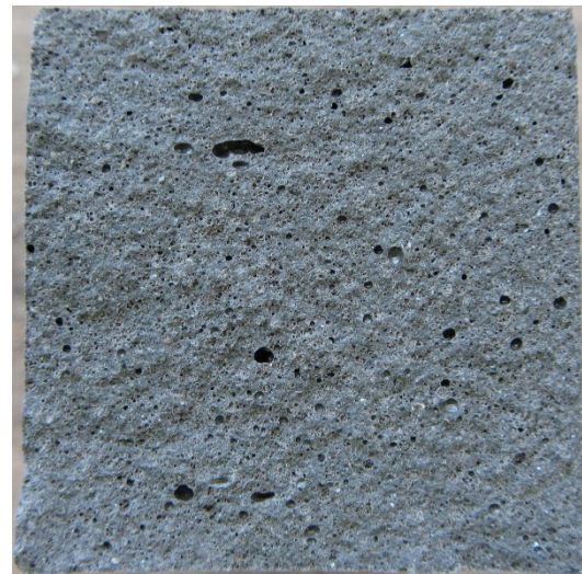
Fig. 16: Photograph of the fracture surface of a prism after bending tensile test
