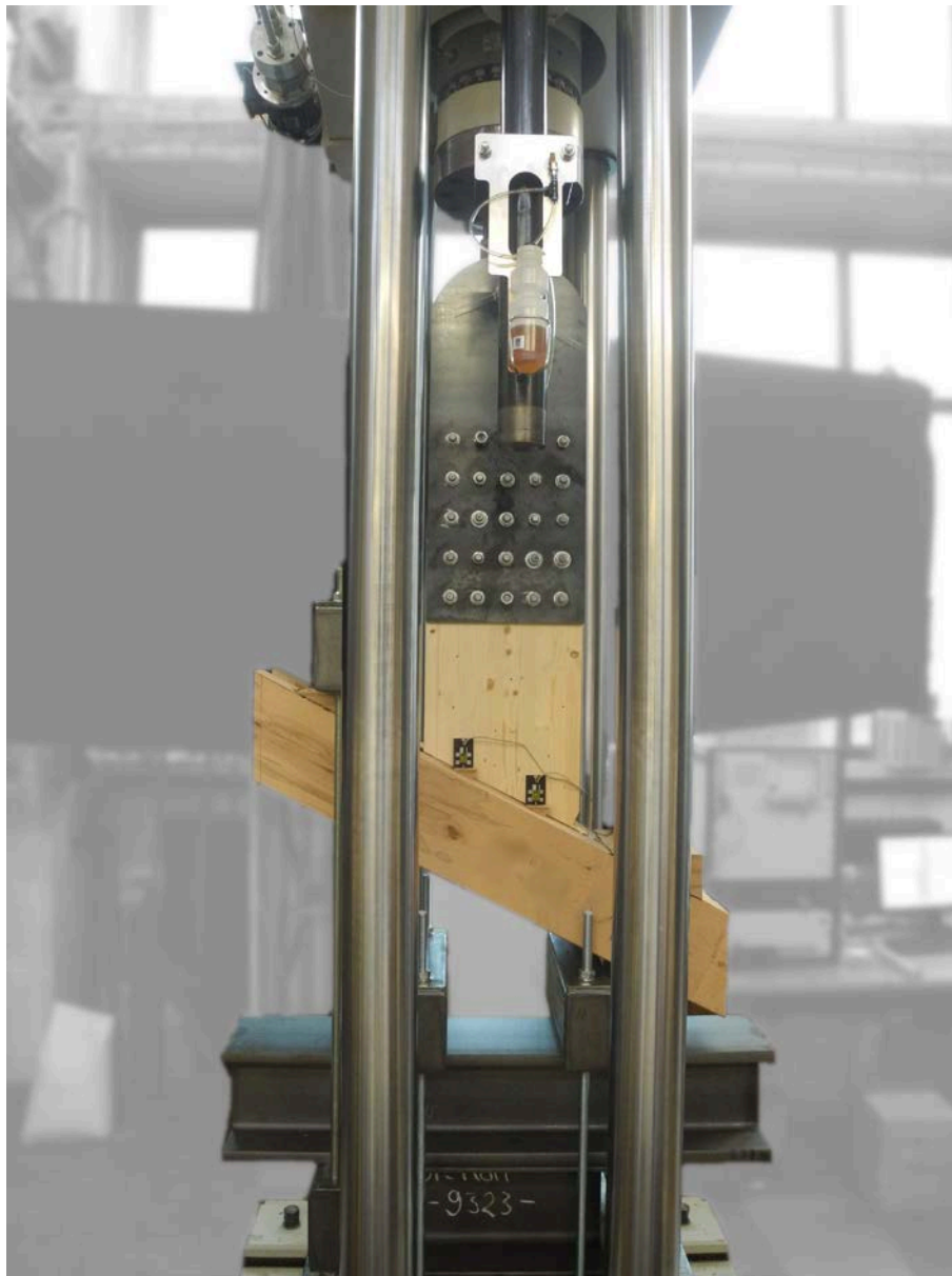
Fig. 2: View of realized experimental test set-up for the tension shear tests
