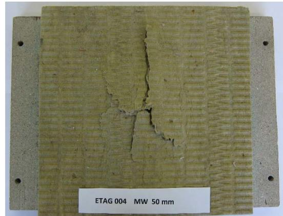
*Fig. 9: Upper side of 50 mm test specimen*
