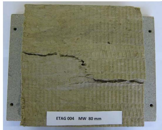
*Fig. 11: Upper side of 80 mm test specimen*
