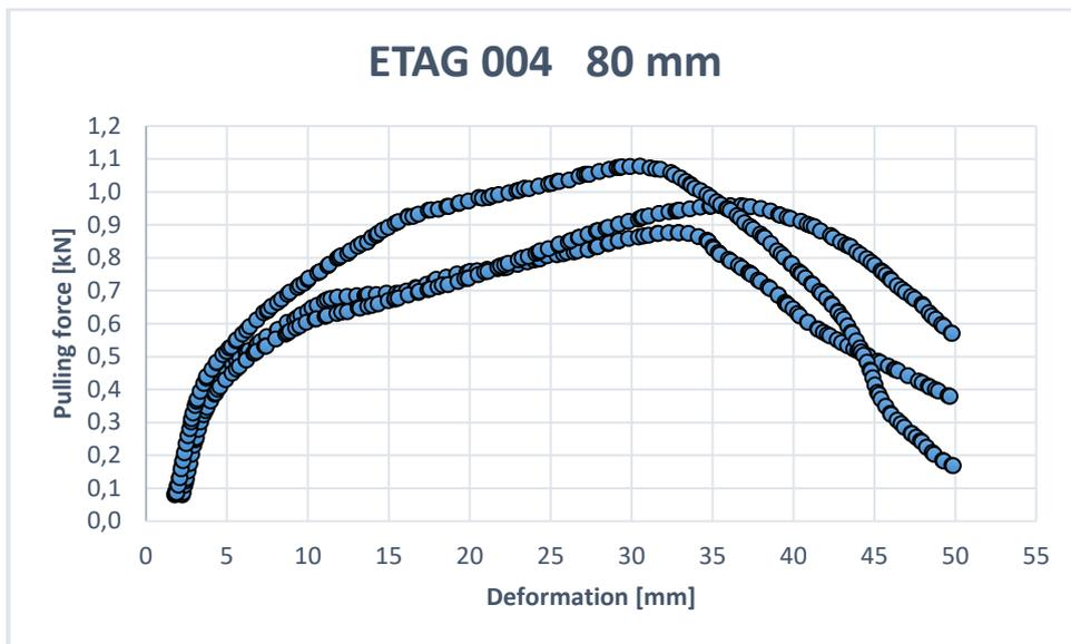
Fig. 3: Force-strain curve of 80 mm thick MW board type 2
