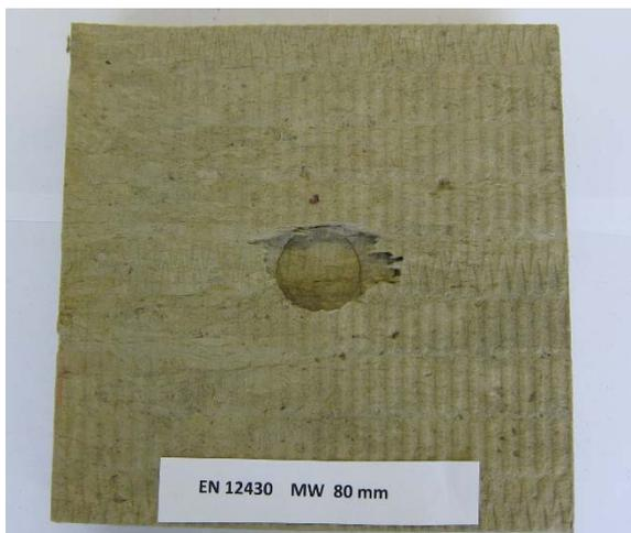
*Fig. 18: Lower side of 80 mm test specimen*
