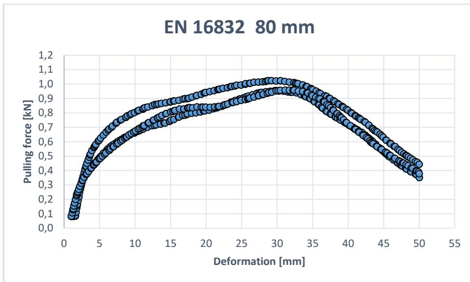
*Fig. 5: Force-strain curve of 80 mm thick MW board type 2*
