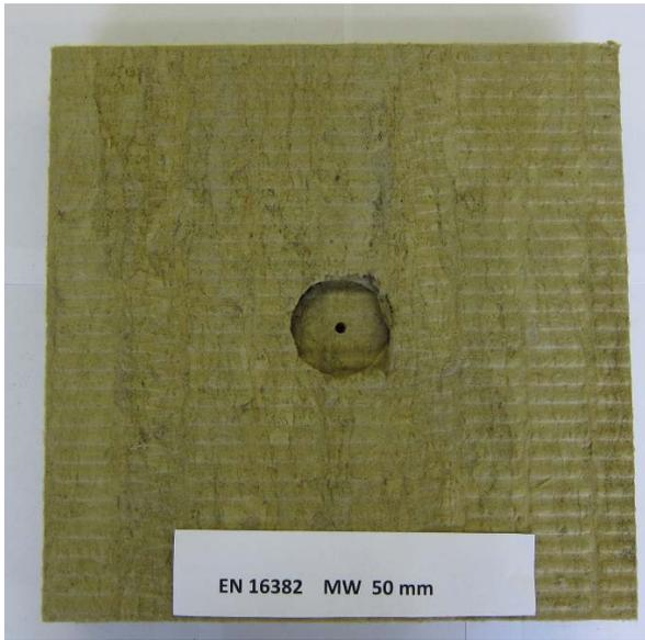
*Fig. 12: Lower side of 50 mm test specimen*
