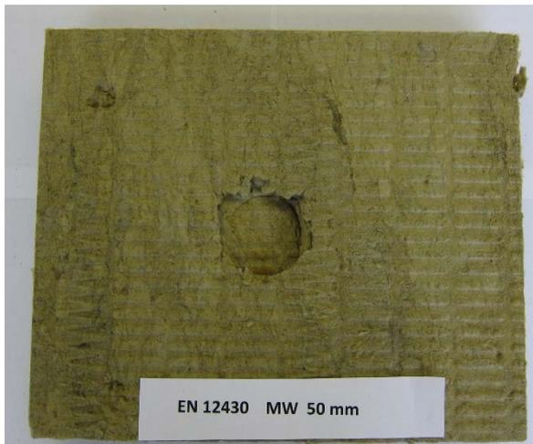
*Fig. 16: Lower side of 50 mm test specimen*
