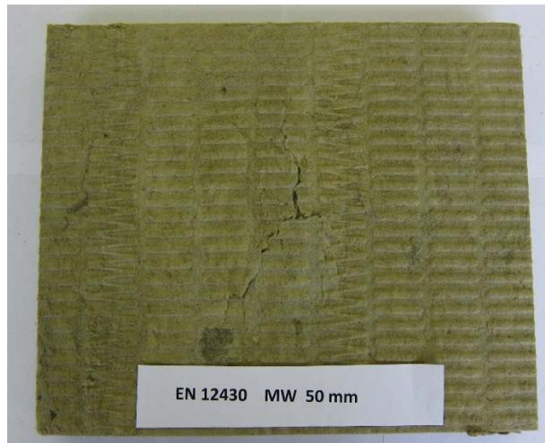
*Fig. 17: Upper side of 50 mm test specimen*
