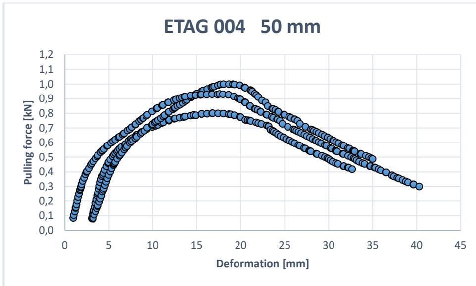
Fig. 2: Force-strain curve of 50 mm thick MW board type 1
