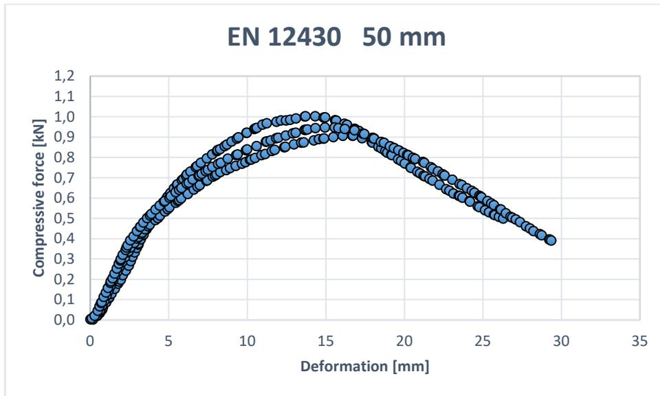
Fig. 6: Force-strain curve of 50 mm thick MW board type 1
