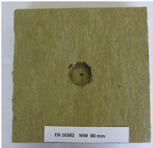
*Fig. 14: Lower side of 80 mm test specimen*
