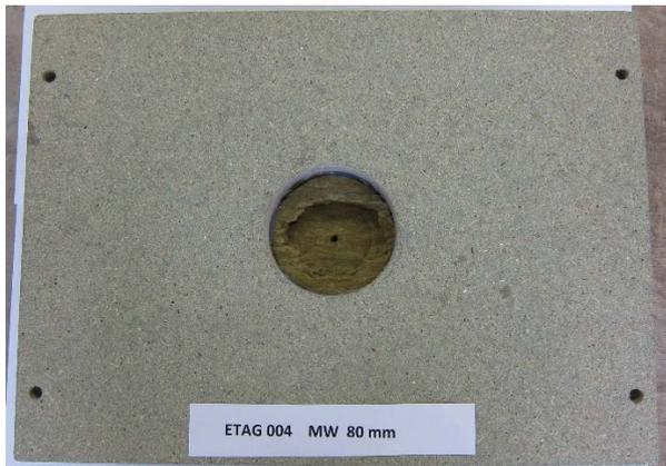
*Fig. 10: Lower side of 80 mm test assembly*
