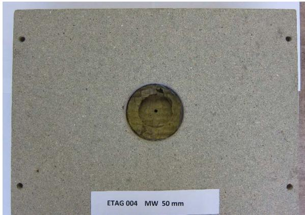
*Fig. 8: Lower side of 50 mm test assembly*
