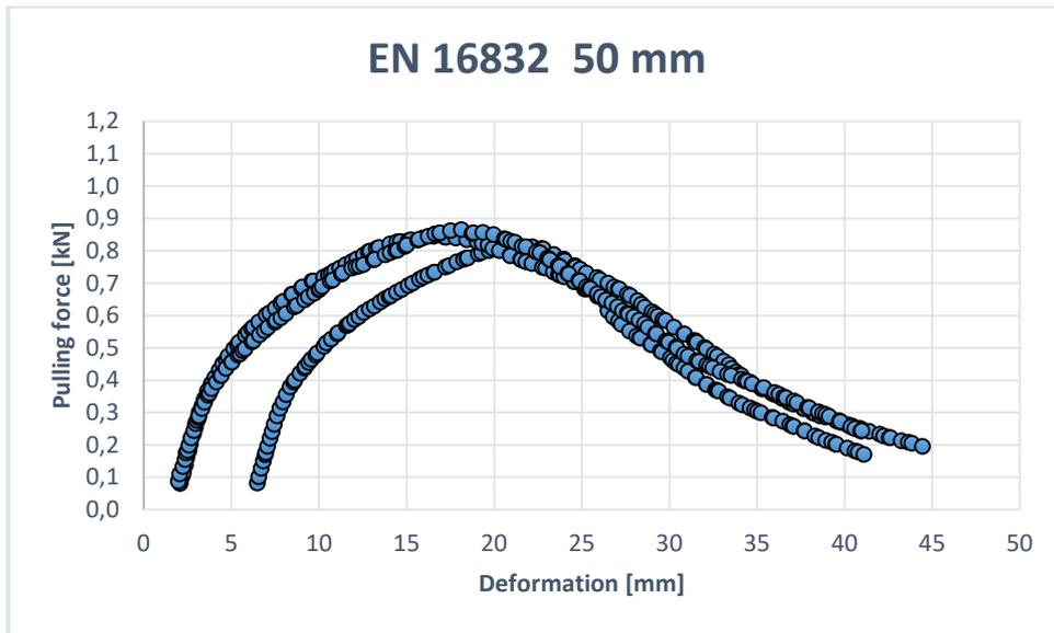
*Fig. 4: Force-strain curve of 50 mm thick MW board type 1*
