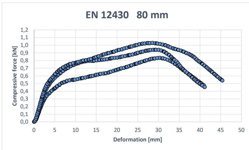
Fig. 7: Force-strain curve of 80 mm thick MW board type 2
