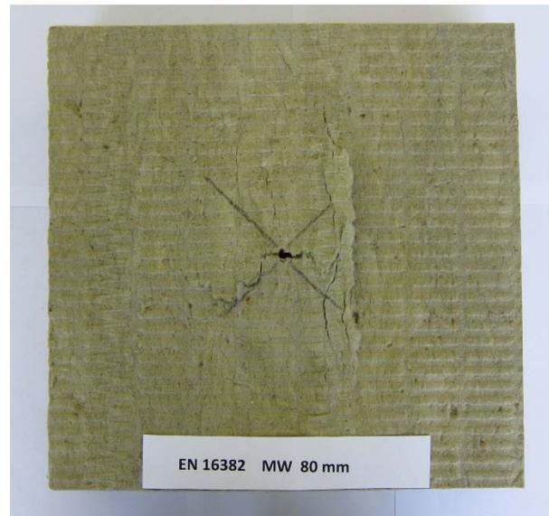
*Fig. 15: Upper side of 80 mm test specimen*
