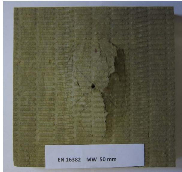
*Fig. 13: Upper side of 50 mm test specimen*
