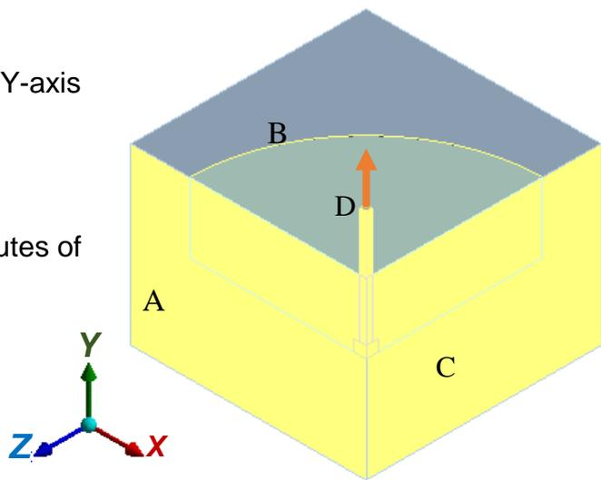
Fig. 4: Boundary conditions for thermal stress analysis
