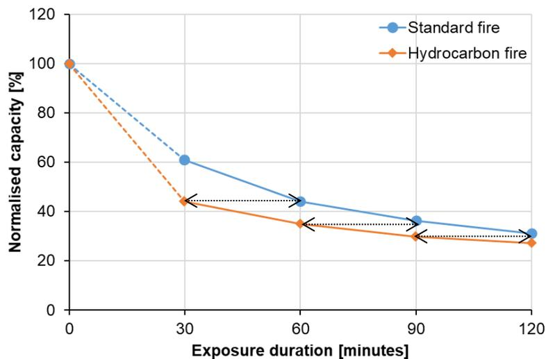
Fig. 8: Predicted reduction of concrete cone capacity for standard fire and hydrocarbon fire exposure
