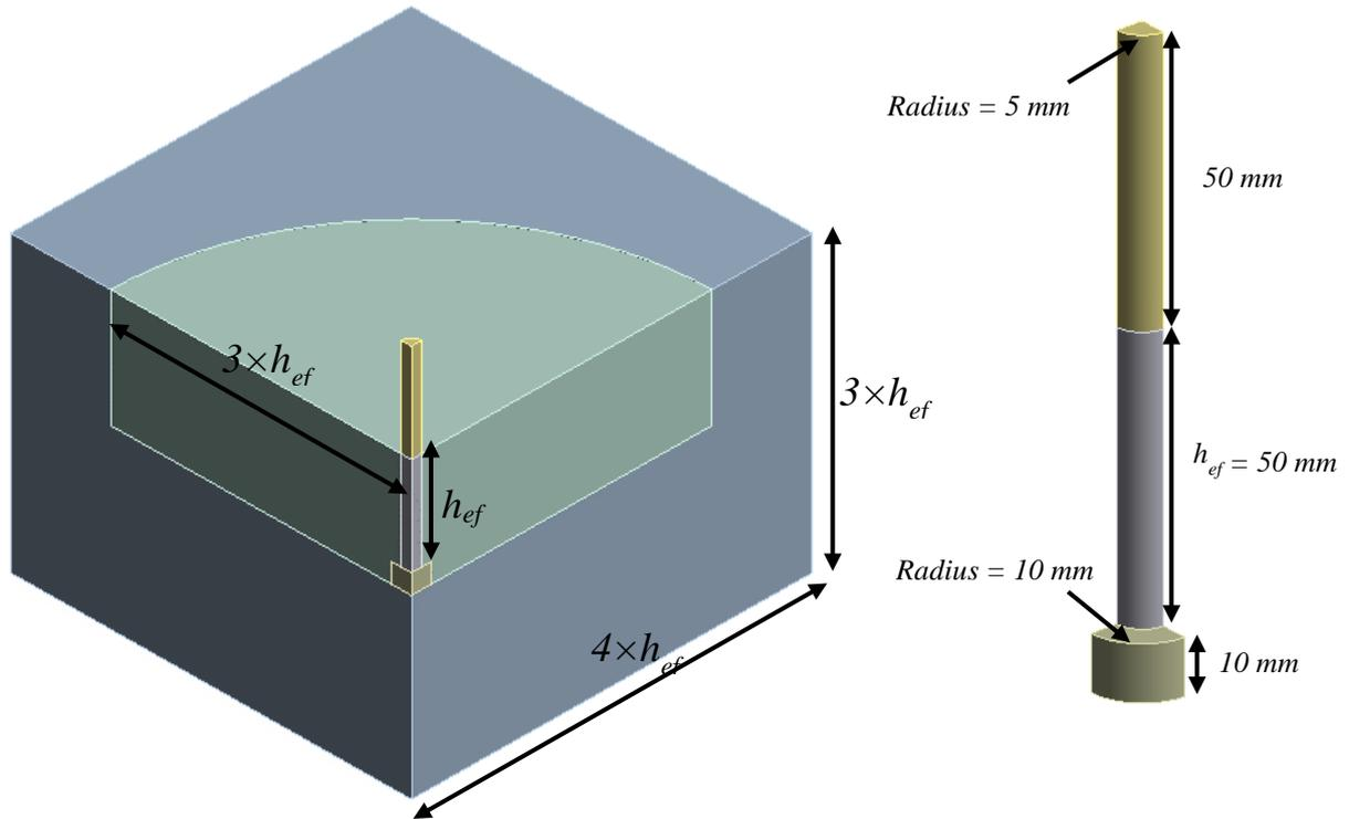
Fig. 1: Geometric details of the headed stud and the concrete volume
