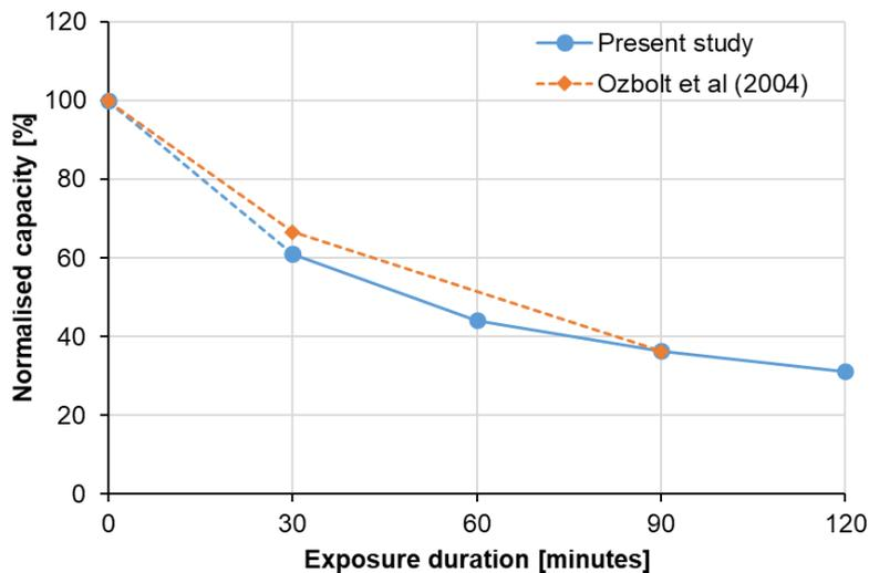
*Fig. 7: Comparison between results predicted in this study and those from literature (for standard fire exposure only)*
