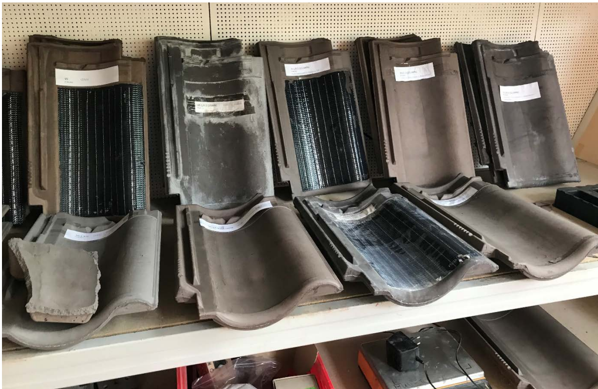
Fig. 6: Material developments for finding the suitable compound composition, color shade and for integrating the PV laminates - test series
