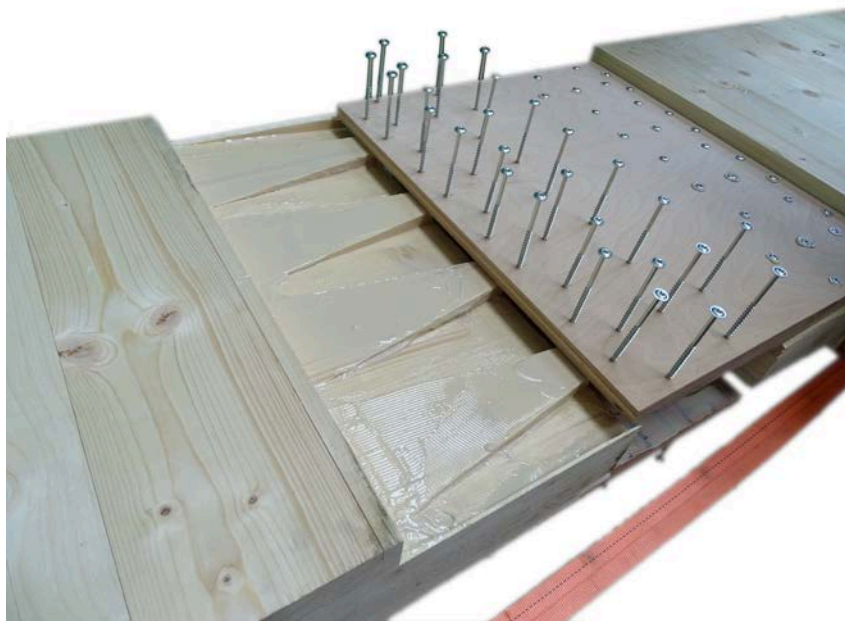
Fig. 4: View of profiles CLT surfaces of connection alternative B and second step of joint assembly by screw gluing
