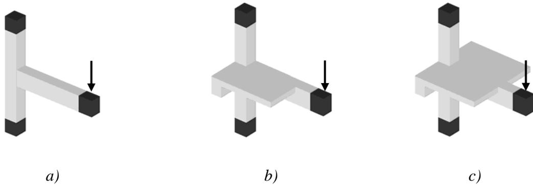
Fig. 3: Investigated exterior beam-column joints: a) 2D joint, b) corner joint and c) edge joint
