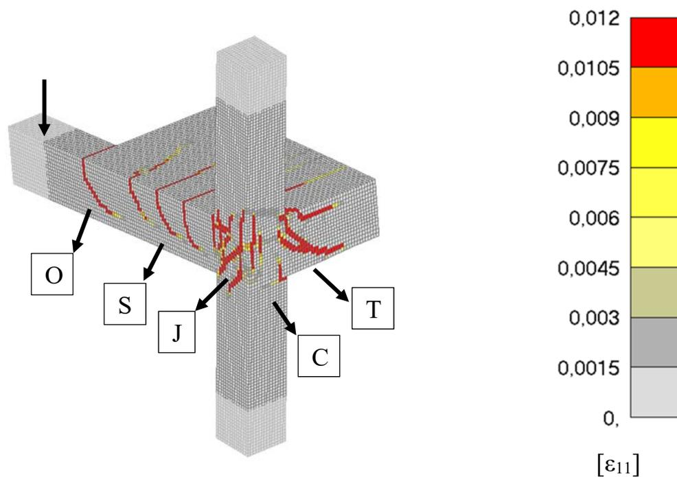
Fig. 5: Description of different cracking stages on corner joint at failure
