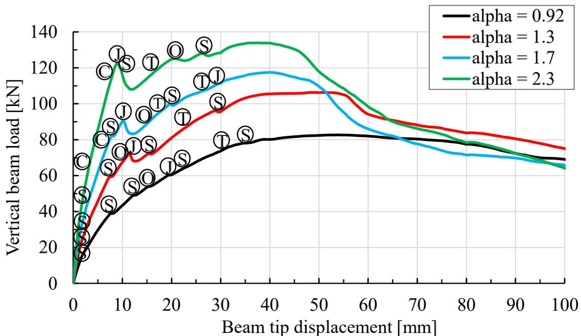
Fig. 8: Load-displacement curves of the corner beam-column joints
