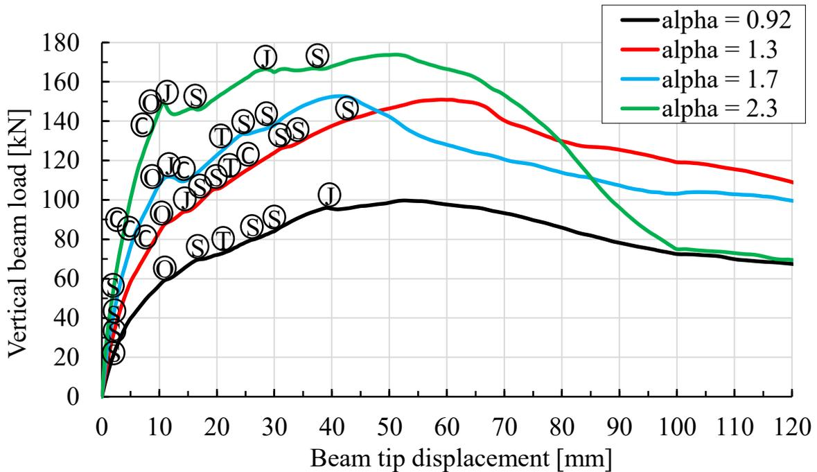
Fig. 10: Load-displacement curves of the edge beam-column joints
