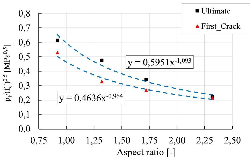
Fig. 9:  $p_t$  versus alpha of the corner beam-column joints
