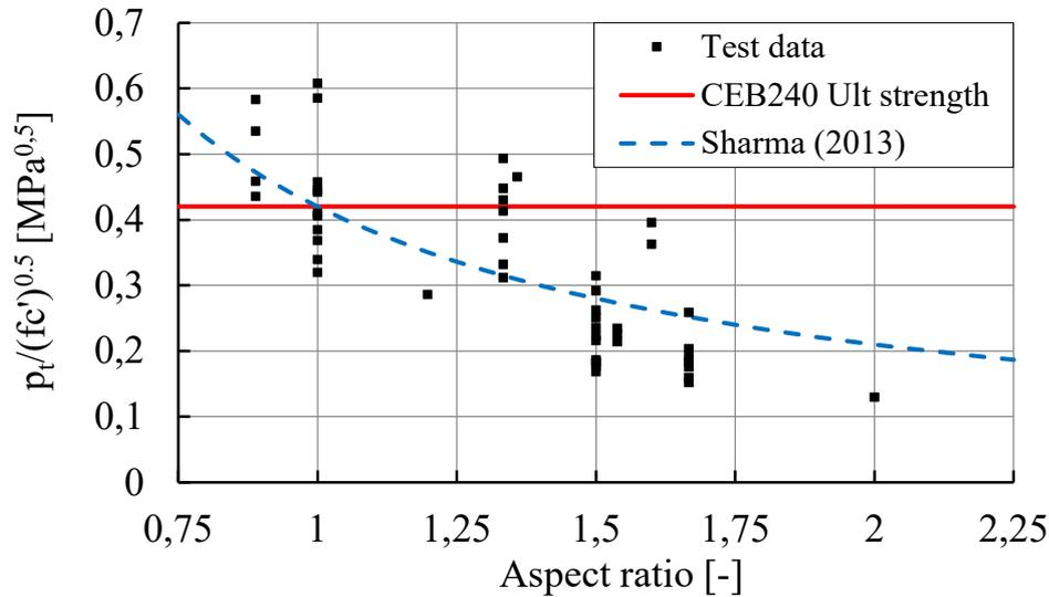
Fig. 1: Data base of exterior joints with bent in longitudinal beam bars
