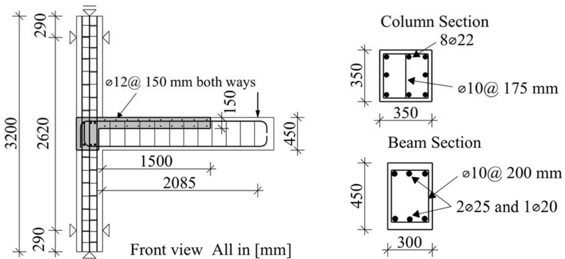
Fig. 4: Geometry and reinforcement detailing of the investigated beam-column joints
