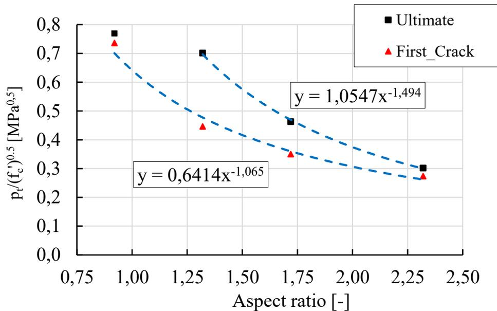
Fig. 11:  $p_t$  versus  $\alpha$  of the edge beam-column joints
