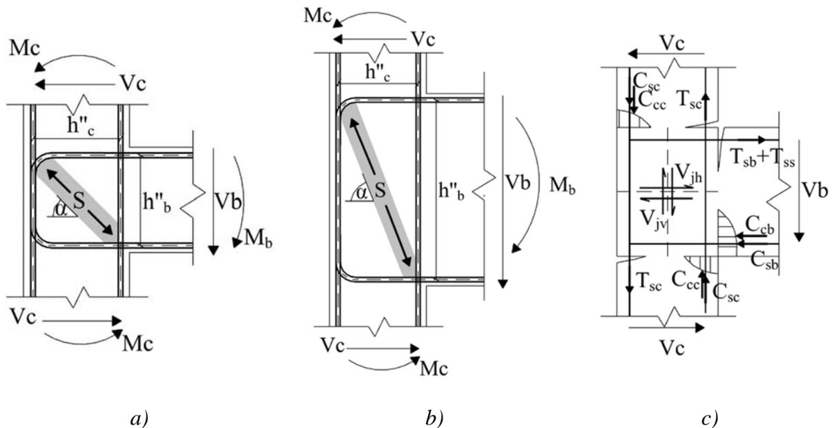
Fig. 2: Diagonal strut formation for a) alpha = 1, b) alpha = 2 and c) horizontal and vertical joint shear of an exterior beam-column joint with slab
