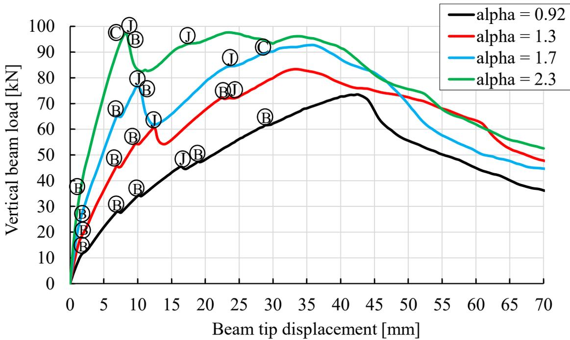
Fig. 6: Load-displacement curves of the 2D beam-column joints
