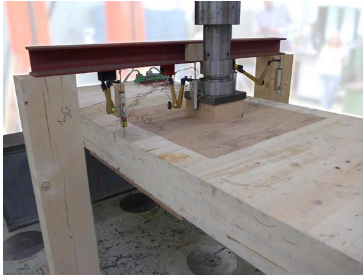
Fig. 9: Realized test set-up with the developed plate-column connection
