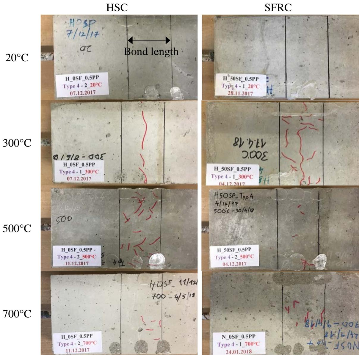
Fig. 8: Typical failure patterns - pull-out tests for specimens with rebar in the center
