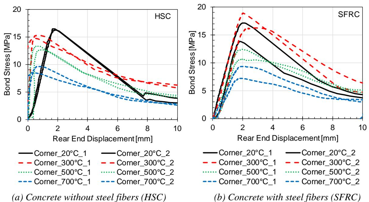
Fig. 7: Bond stress-slip curves - pull-out tests on specimens with rebar in the corner
