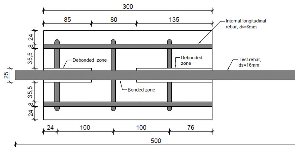
Fig. 1: Typical reinforcement detailing of the test specimen
