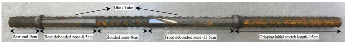
Fig. 3: Test rebar with glass tubes
