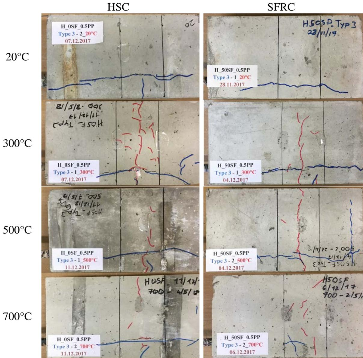
Fig. 10: Typical failure patterns from pull-out tests for specimens with rebar in the corner
