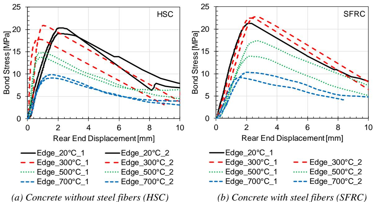
Fig. 6: Bond stress-slip curves obtained - pull-out tests on specimens with rebar at the edge
