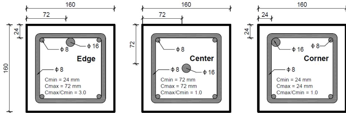
Fig. 2: Positions of test rebar investigated in the test program
