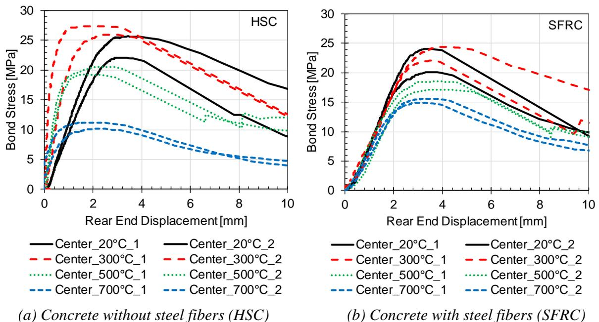
Fig. 5: Bond stress-slip curves obtained - pull-out tests on specimens with rebar in the center
