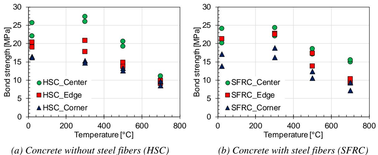
Fig. 11: Bond strength as a function of temperature for different specimens
