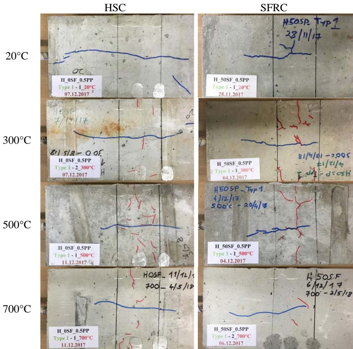
Fig. 9: Typical failure patterns - pull-out tests for specimens with rebar at the edge
