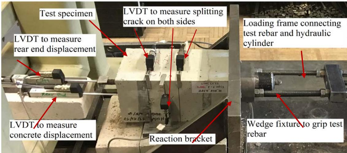
Fig. 4: Test setup employed for performing pull-out tests
