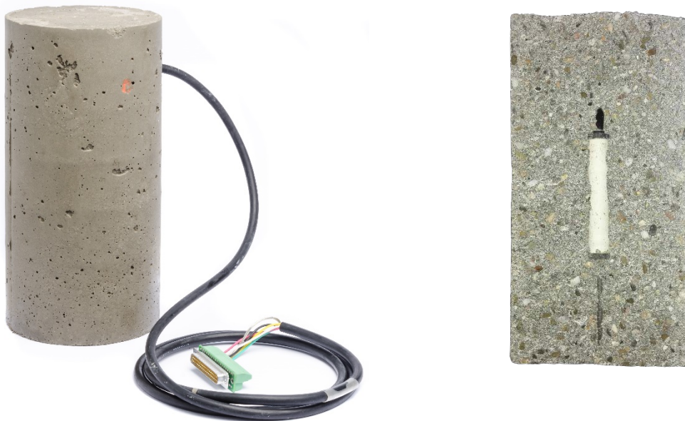
Fig. 3: Cylinder for creep test (left) and split cylinder showing interior Linear Voltage Differential Transformers (LVDT) for creep test (right) (source: [2]).
