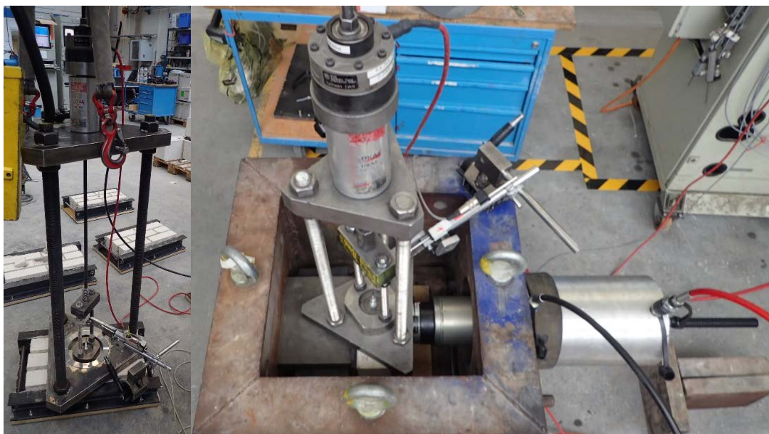
Fig. 2: Test setup for stretcher bond and test setup for clamped NF brick
