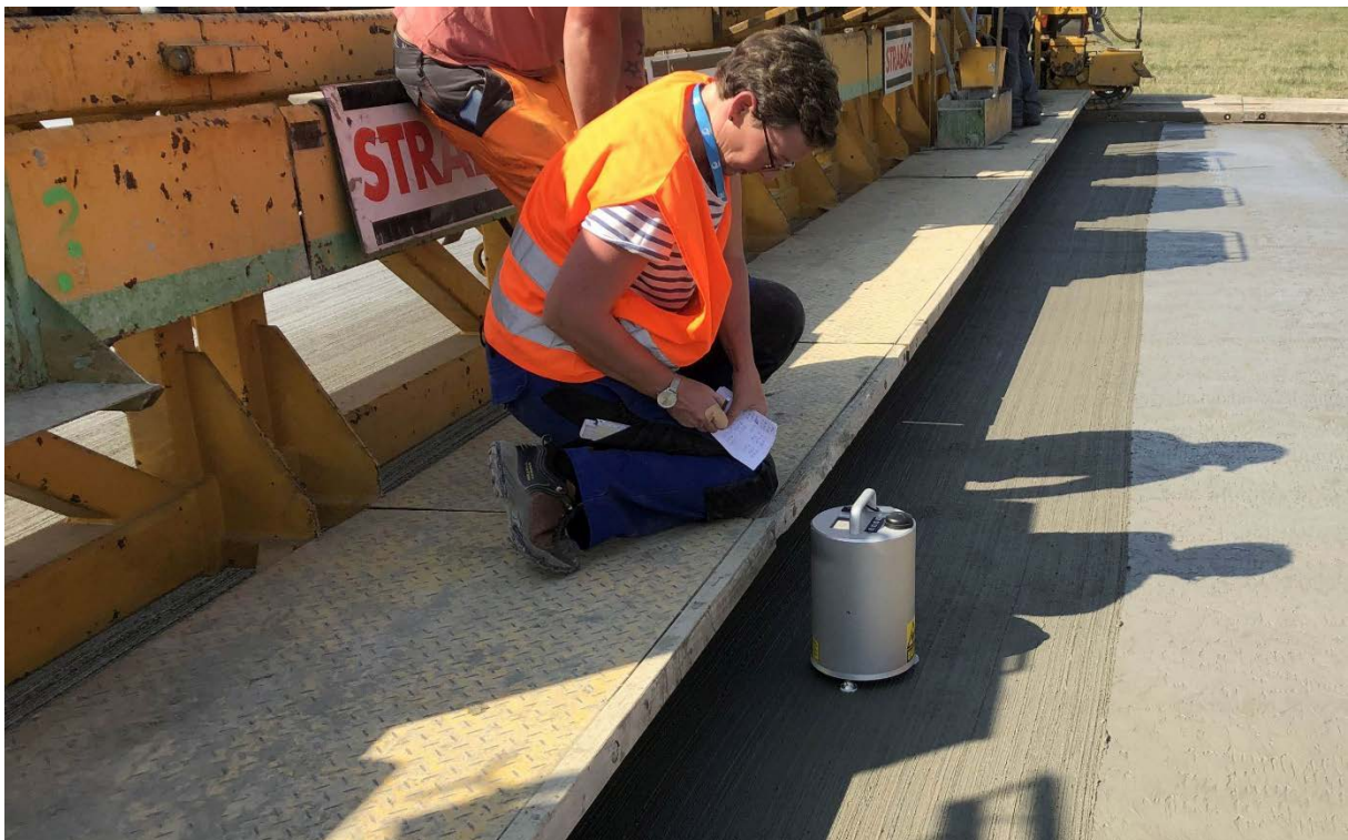
Fig. 11: Measurement on the concrete surface with a laser-based texture depth meter
