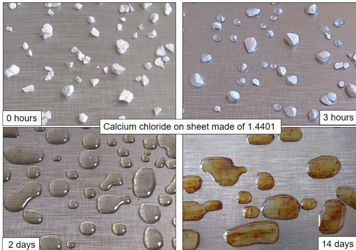
Fig. 2: Liquefaction of calcium chloride on sheet steel 1.4401 in dry air ( \approx 45\% relative air humidity) (Source: Lecture Nürnberg)
