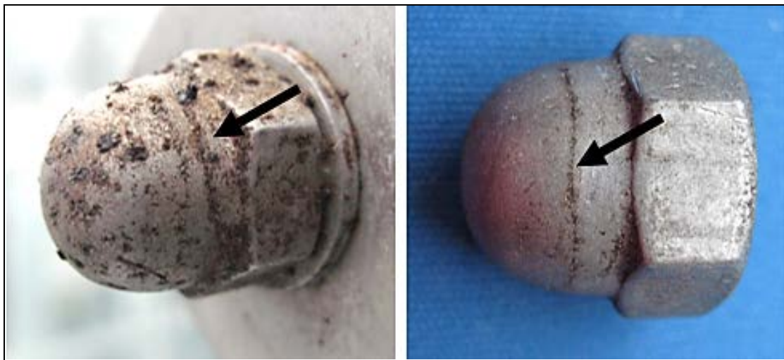
Figs. 10 and 11: Stress corrosion cracking of welded joint on tension bars made of stainless steel 1.4571 after 9 years
