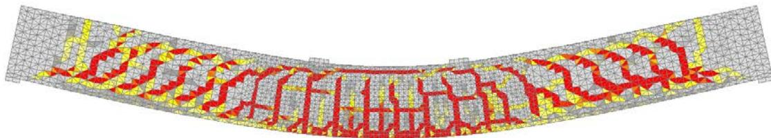
(b) Section along the length of the beam without lap splice at failure (LL2)
