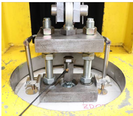
(a) Undercut anchor
