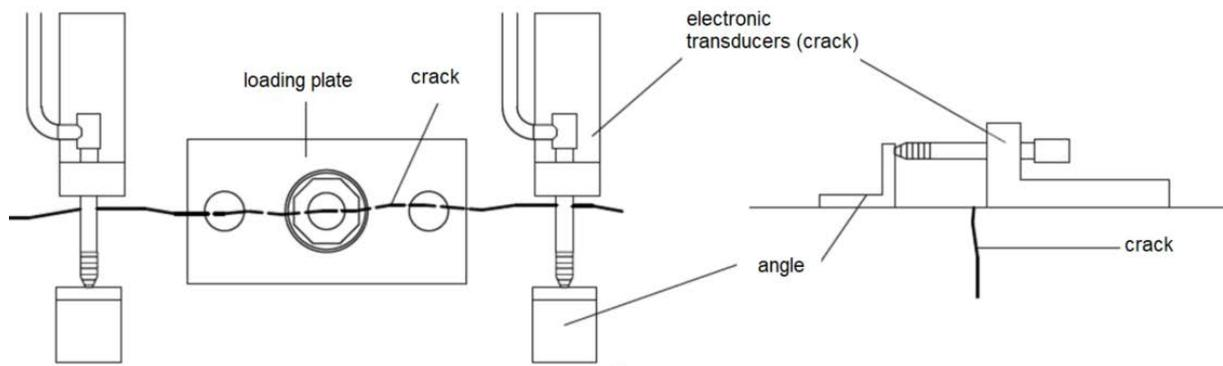
Fig. 4: Arrangement of the crack sensors for measuring the crack displacement
