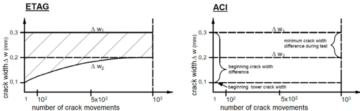
Fig. 1: Different representation of the allowable crack opening variations during the crack movement test (Functioning in crack movement) according to [1, 2]
