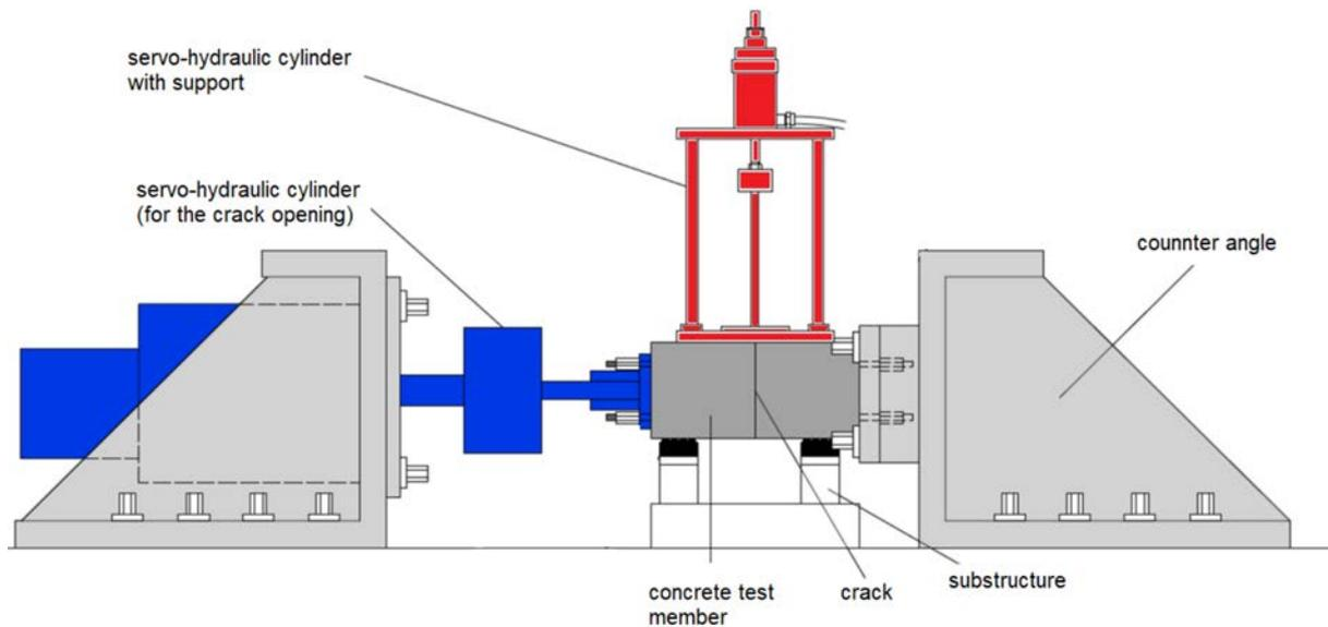
*Fig. 2: Schematic representation of the loading setup for fasteners under static load with repeated crack opening*
