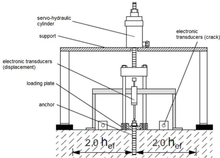
Fig. 3: Loading setup for tensile tests away from edges in cracked concrete according to [3]
