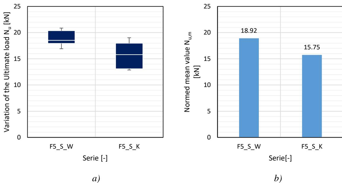
Fig. 9: Normalized ultimate loads with variation a) and mean value b) in tests with concrete screws
