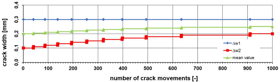
Fig. 5: Illustration of crack opening with displacement-controlled crack
