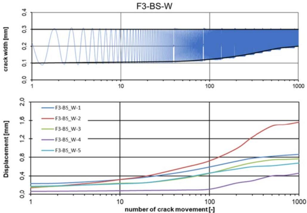
Fig. 6: Crack widths and fasteners displacements of the tests with concrete screws under displacement-controlled crack opening
