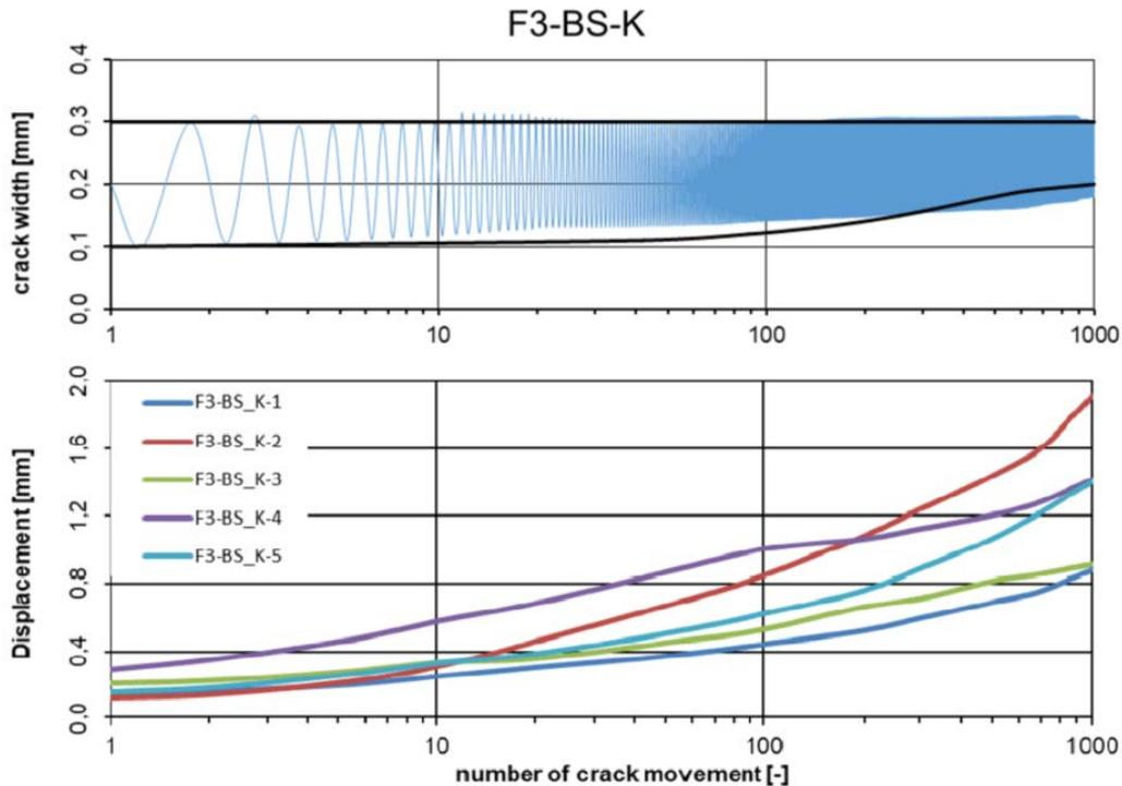
Fig. 7: Crack widths and fasteners displacements of the tests with concrete screws under load-controlled crack opening
