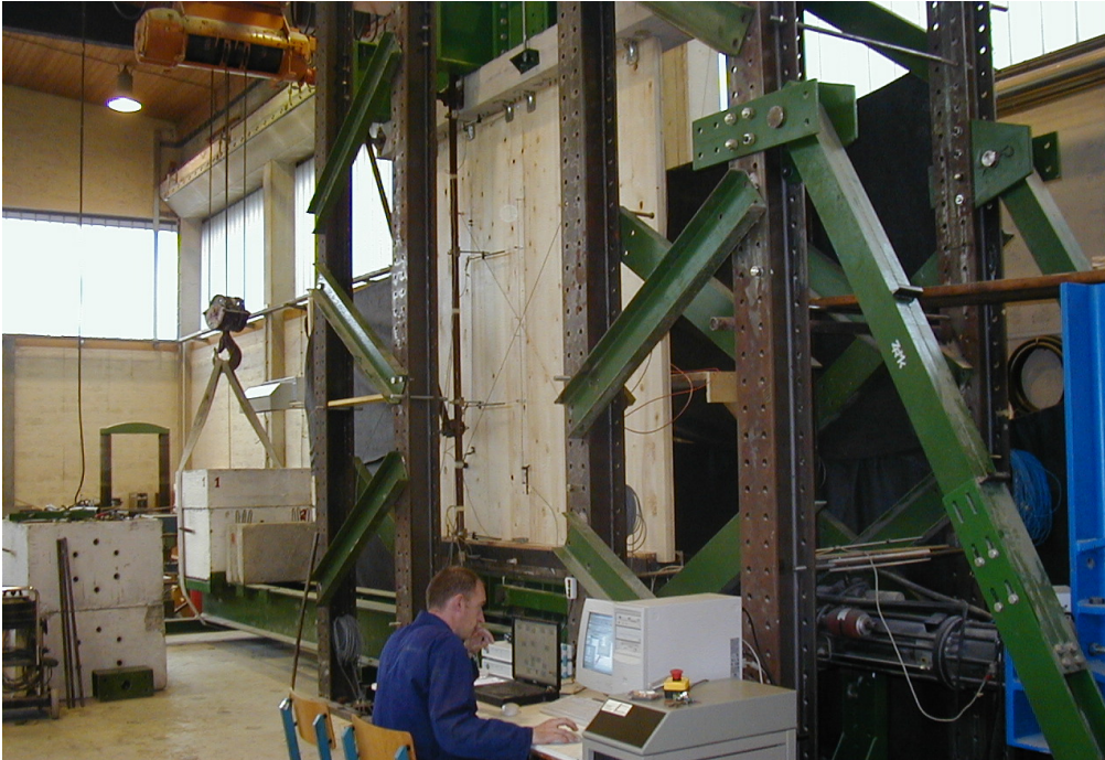
Figure 4: Setup for cycling testing of panels
