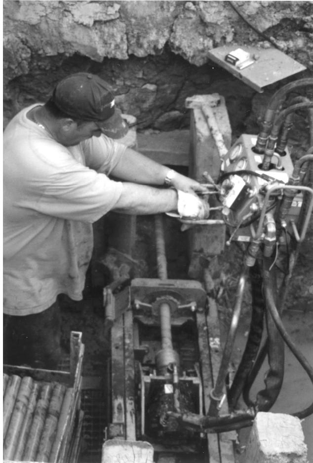
Figure 4: One example of Horizontal Directional Drilling equipment for small drilling diameters up to 110 mm (with a reamer up to 150 mm) and drilling distances up to 50 m (Tracto-Technik Comp., frame rig, syst. Grundopit). Drilling tests in Stuttgart-Vaihingen, July 2006
