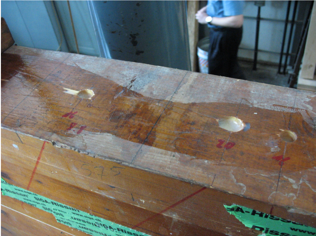
Figure 2: View of glued-in rods at the support
