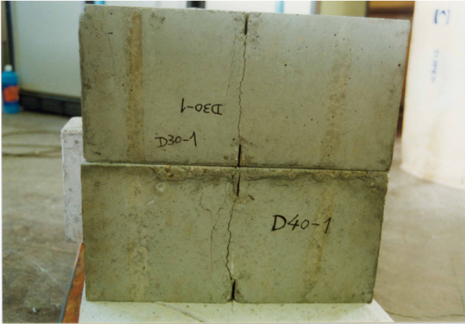
Figure 20. Crack pattern of two specimens from series D with 30 and 40 mm deep notches
