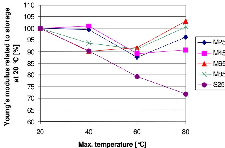
Fig. 12: Percentage difference in the Young's modulus of the powder types and the viscosity-agent type related to standard storage at an effective age of 3 d and different maximum curing temperatures
