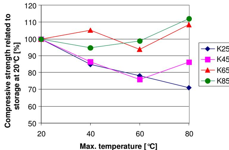
Fig. 2: Percentage difference in the compressive strength of the combination types related to standard storage at an effective age of 3 d and different maximum curing temperatures
