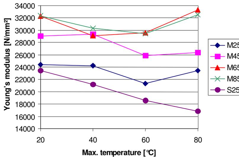
Fig. 11: Comparison of the Young's modulus of the powder types and the viscosity-agent type at an effective age of 3 d and different maximum curing temperatures
