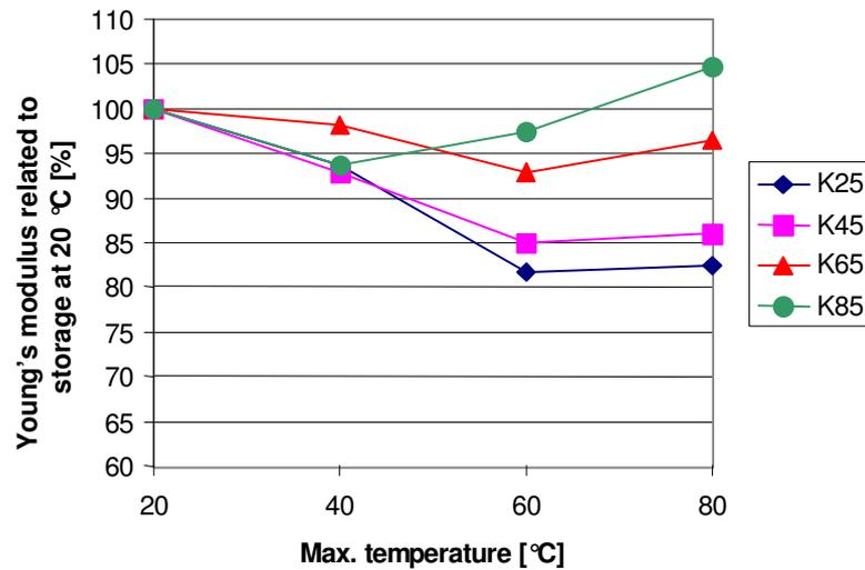
Fig. 10: Percentage difference in the Young's modulus of the combination types related to standard storage at an effective age of 3 d and different maximum curing temperatures
