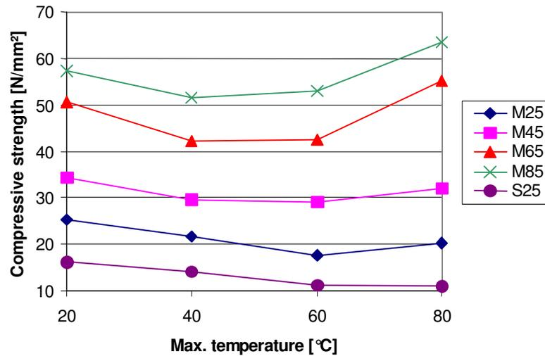
Fig. 3: Comparison of compressive strengths of the powder types and the viscosity-agent type at an effective age of 3 d and different maximum curing temperatures
