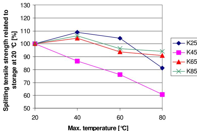
Fig. 6: Percentage difference in the splitting tensile strength of the combination types related to standard storage at an effective age of 3 d and different maximum curing temperatures.
