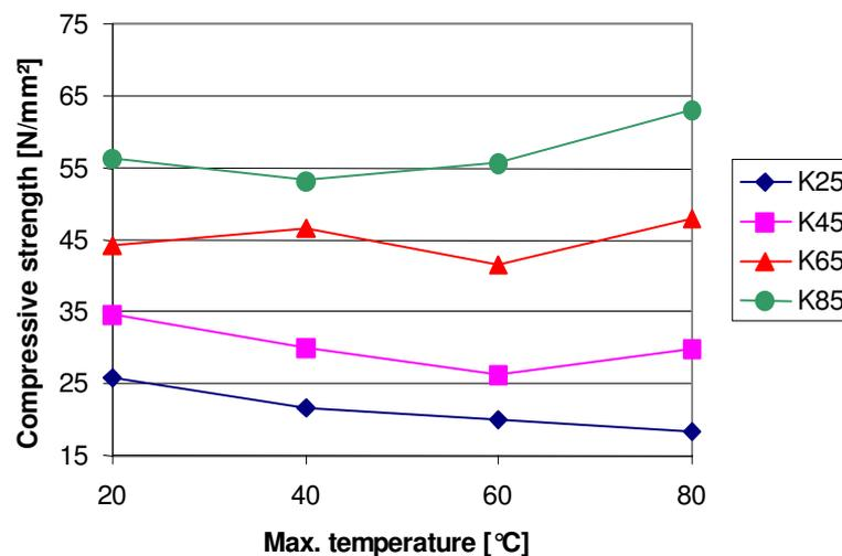
Fig. 1: Comparison of compressive strengths of the combination types at an effective age of 3 d and different maximum curing temperatures
