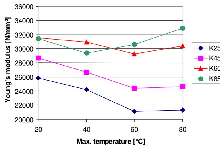
Fig. 9: Comparison of the Young's modulus of the combination types at an effective age of 3 d and different maximum curing temperatures.
