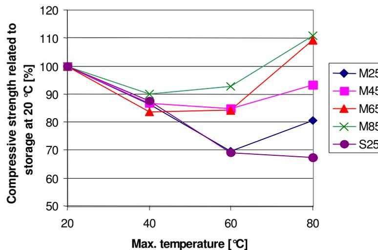
Fig. 4: Percentage difference in the compressive strength of the powder types and the viscosity-agent type related to standard storage at an effective age of 3 d and different maximum curing temperatures
