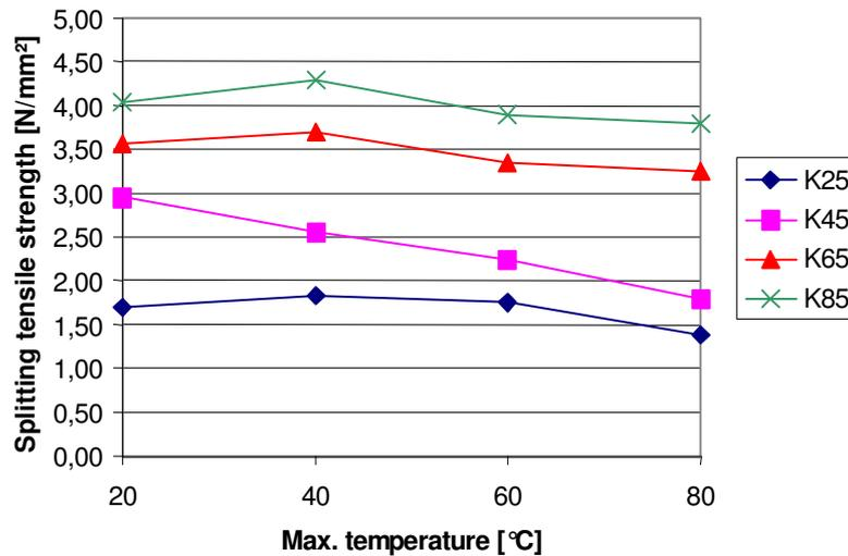
Fig. 5: Comparison of splitting tensile strengths of the combination types at an effective age of 3 d and different maximum curing temperatures.
