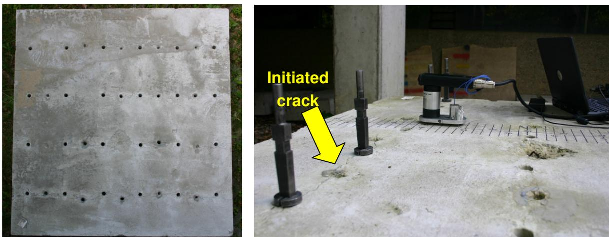
Figure 7. Test specimen for laboratory tests (Cracks initiated by splines)
