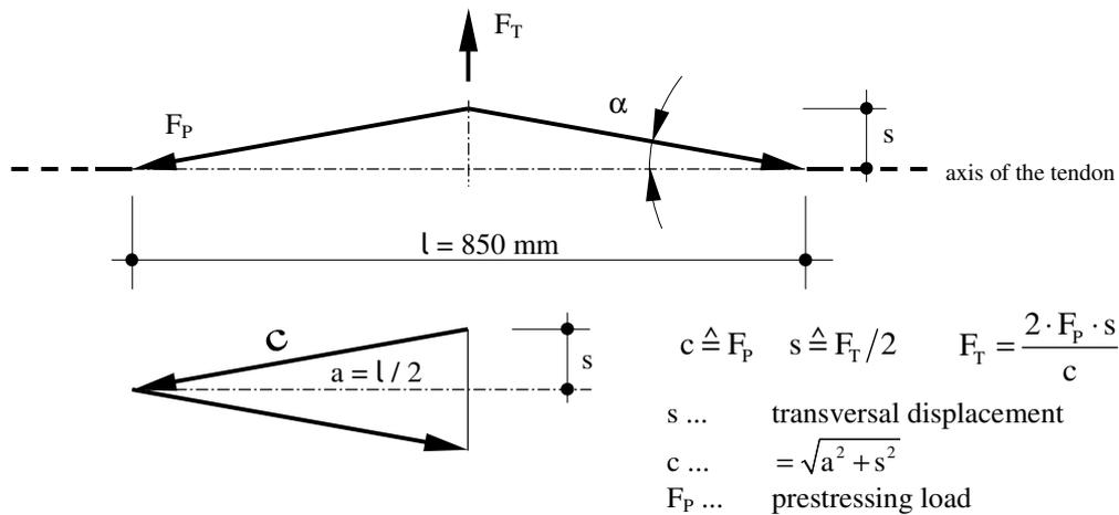
Fig. 6: force-triangle as a result of transversal displacement of the tendon by the tensiometer proceq
