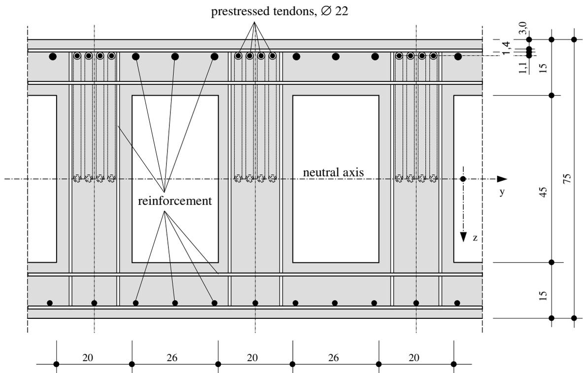
Fig. 3: cross section of the slab
