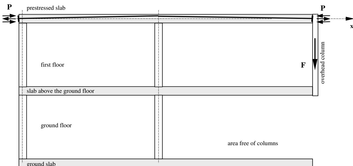
Fig. 1: longitudinal section of the building
