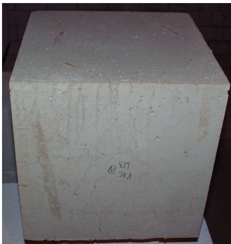
Figure 6: cube 3 of mix K55/67 after fire
