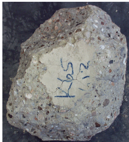
Figure 7: cube 3 of mix K55/67 after brushing off the loose parts.
