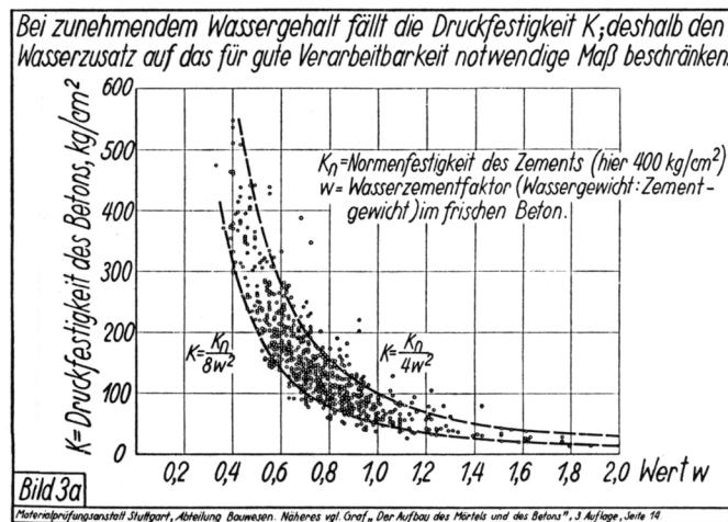
Fig. 3. Compressive strength of concrete as function of the water-cement ratio
