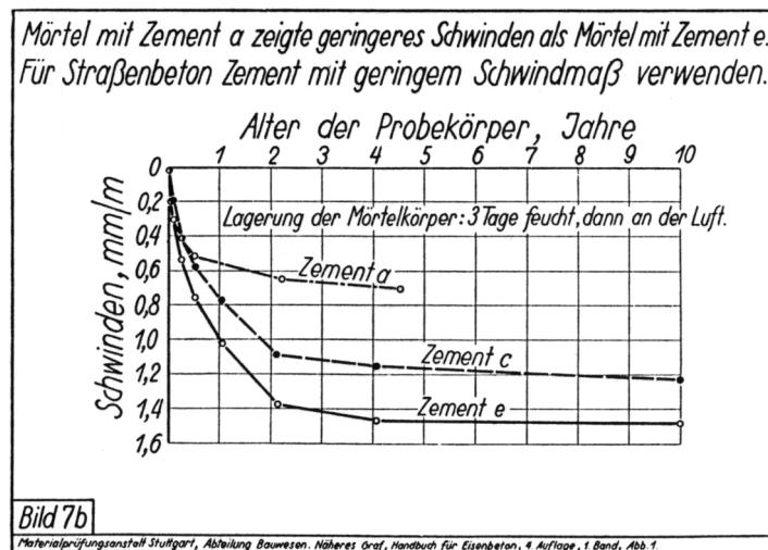
Fig. 5. Shrinkage of various cements [8]
