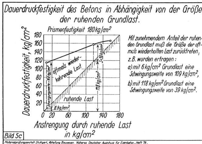
Fig. 4. Goodman-diagram of concrete [8]
