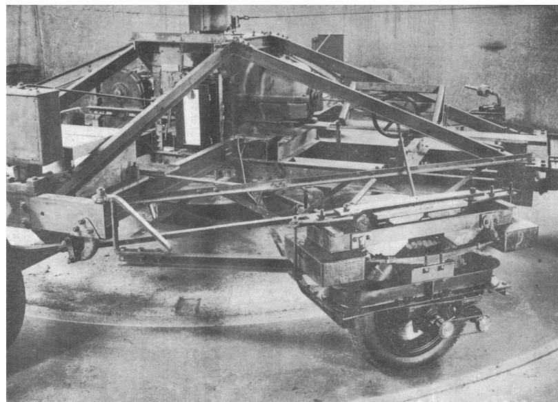
*Fig. 7. Measuring device for the testing of friction between wheel and concrete [19]*
