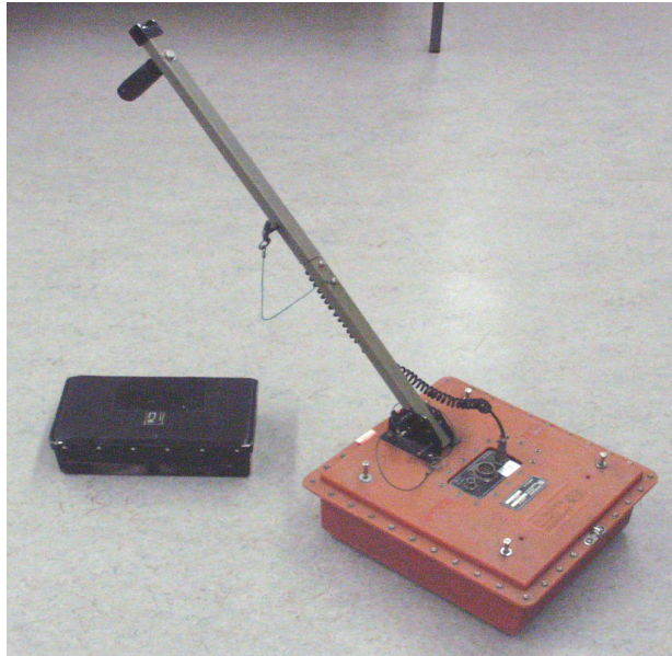
Fig.4: 500 MHz antenna with handle bar and 900 MHz antenna (both by GSSI).
