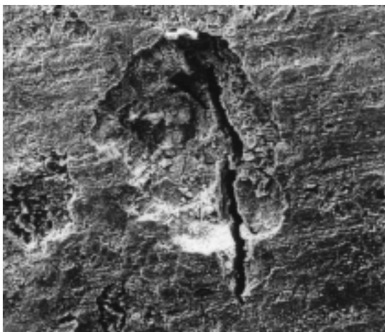
Fig. 3: Pitting induced stress corrosion cracking
