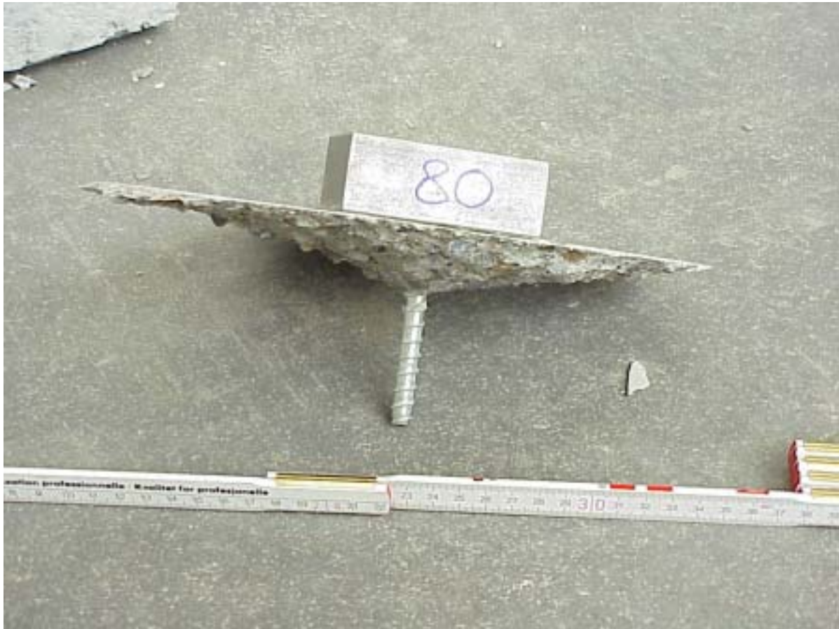
Figure 6: Pull-out cone of a concrete screw
