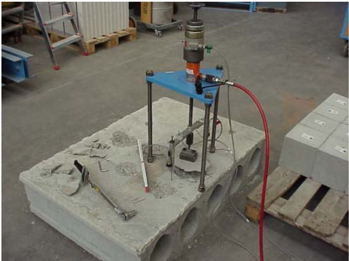
Figure 5: Pull-out tests in a prestressed hollow-cored concrete slab
