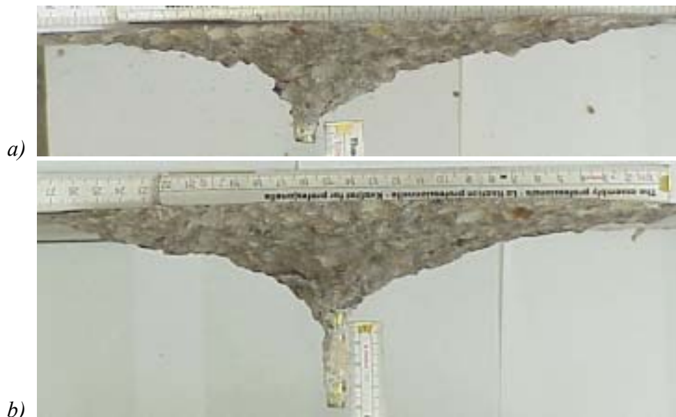
Figure 16: Typical concrete failure cones [9] a) h_{nom} = 50\text{mm} b) h_{nom} = 90\text{mm}
