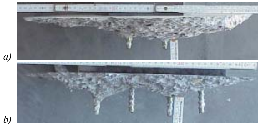
Figure 20: Concrete failure cone of square groups with concrete screws
