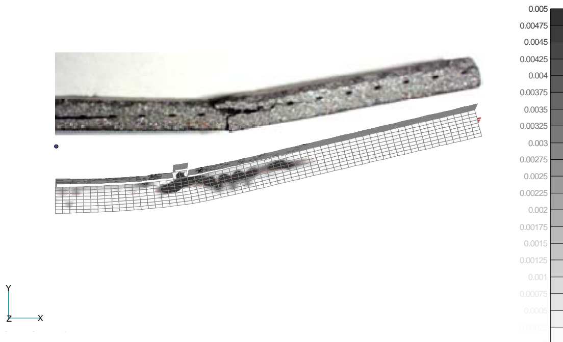
Figure 15: Comparison of tested specimen after test and principle strains of concrete elements in y direction at maximum load.
