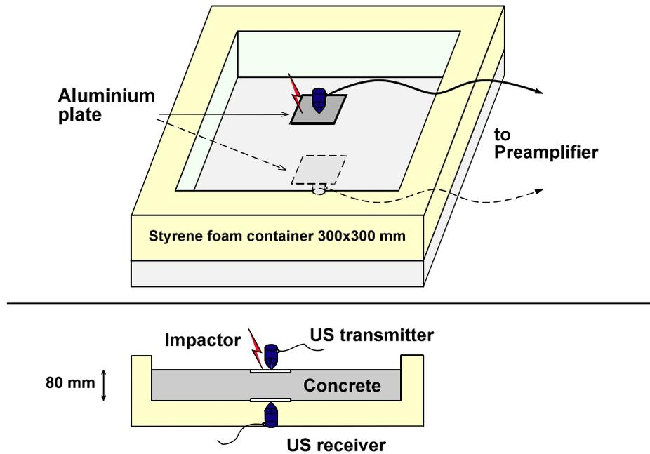
*Fig. 1: Set-up with steel ball impactor and receiver.
