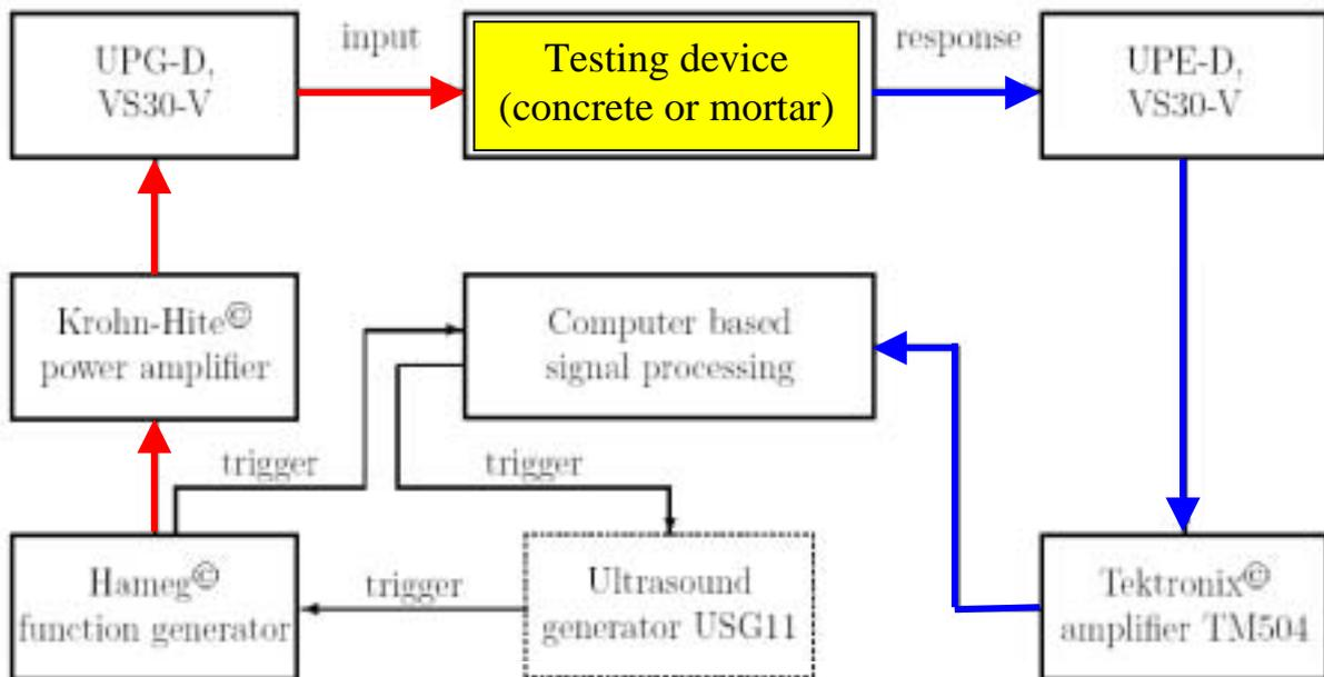
*Fig. 11: Flow chart of newly developed FreshCon experiments.*
