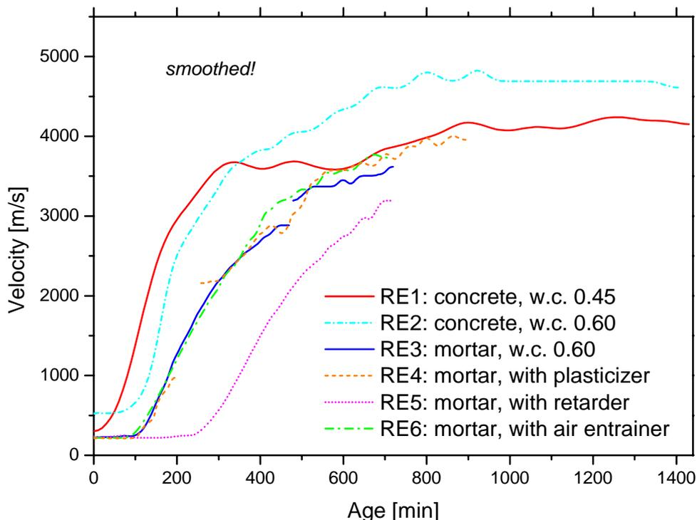
Fig. 13: Comparison of the velocity measurements testing mixtures RE 1-6.
