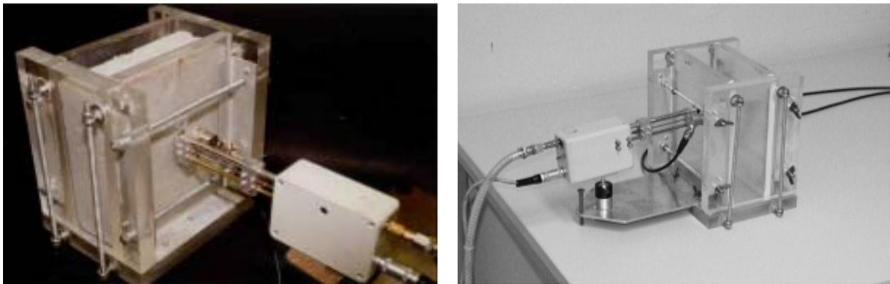
*Fig. 3: Set-up of the first container out of PMMA only.
