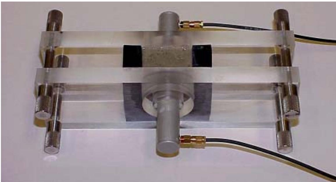
*Fig. 5: Final set-up of the mortar device showing the mould (rubber foam and PMMA-walls) and the transducers.*
