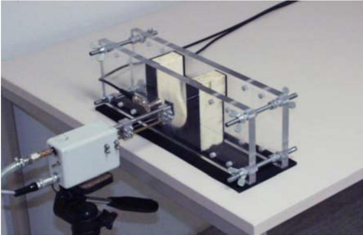
*Fig.6: FreshCon device for concrete measurements developed on the basis of the older mortar device (see Fig.5).*
