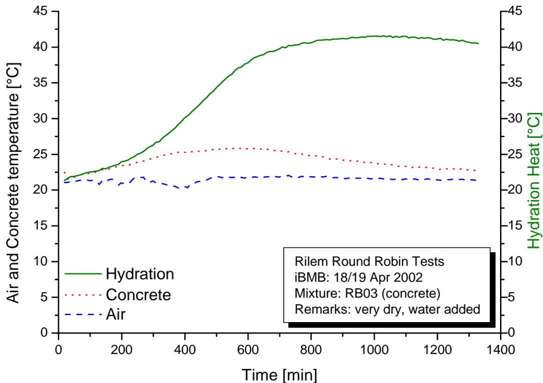
Fig. 9: Results of temperature measurements using the new FreshCon version.
