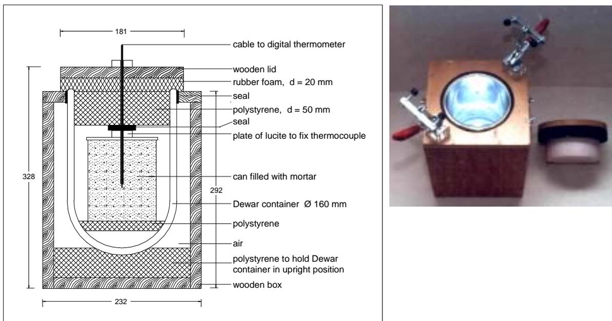
Fig. 8: Set-up of the calorimeter device according KÖBLE [1999], dimensions in mm.
