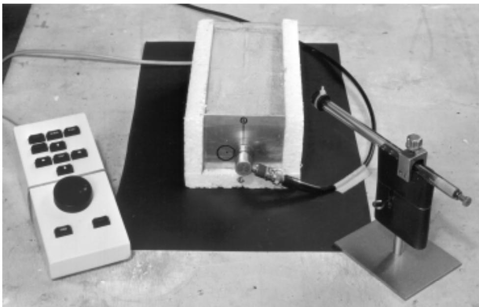
*Fig. 2: Set-up of the smaller styrene foam container with two aluminium side walls.
