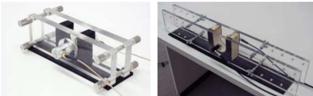
*Fig. 12: Re-designed FreshCon container/sensor for mortar (left) and concrete (right) measurements.*
