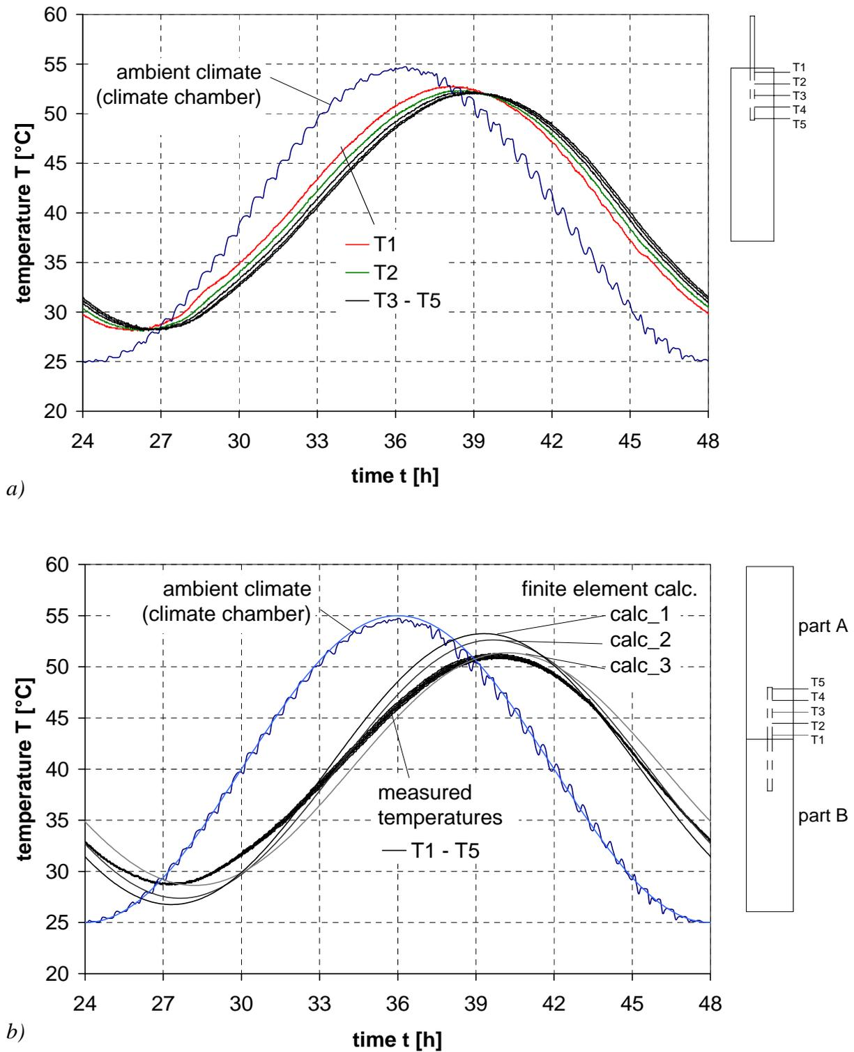
Fig. 6a,b: Temperature evolution over 1 day at a cycle length of 24 hours
