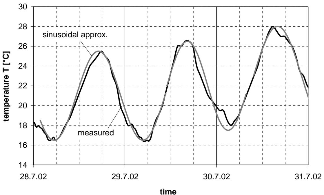
Fig. 3: Course of temperature (sheltered outdoor conditions) of typical summer days and sinusoidal approximation of the temperature
