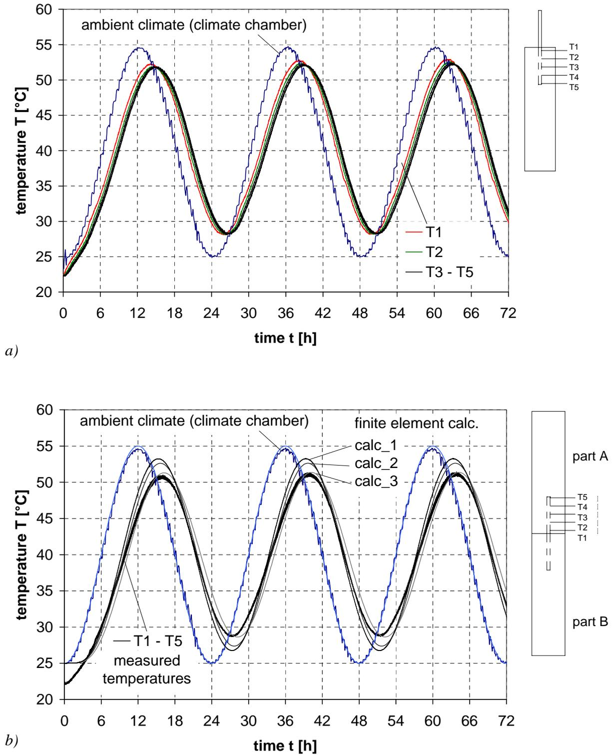
Fig. 5a,b: Temperature evolution over 3 days at the positions of the thermo-elements
