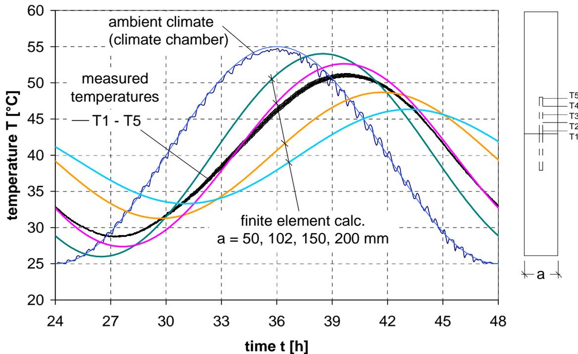
Fig. 7: Temperature evolution at a cycle length of 24 hours for finite element calculations with varying timber thicknesses compared to experimental results (specimen No. II with hidden rod)
