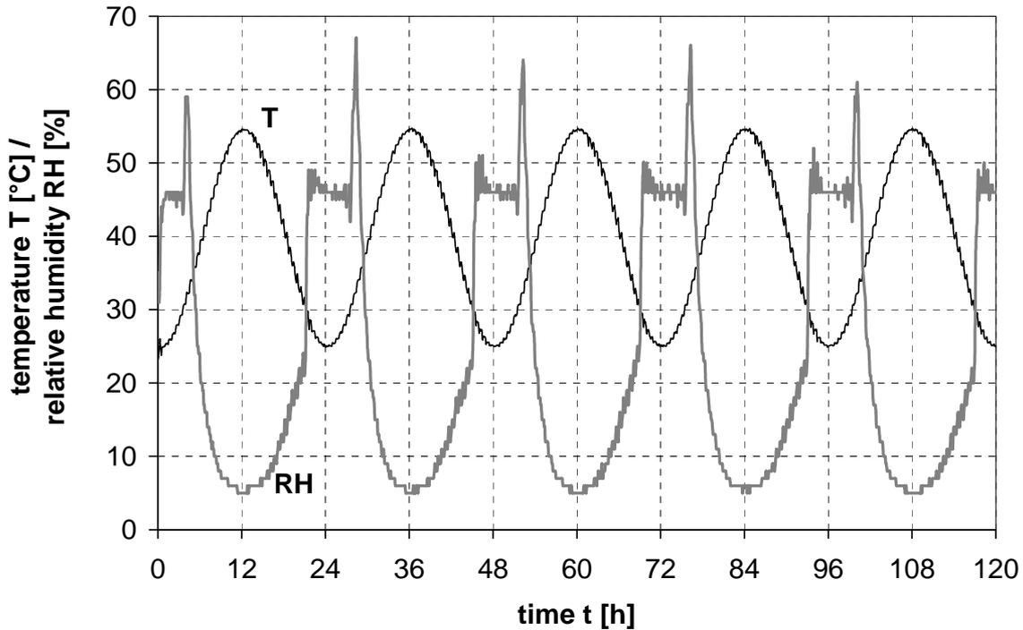
Fig. 4: Course of the applied ambient temperature and relative humidity variation in the climate chamber
