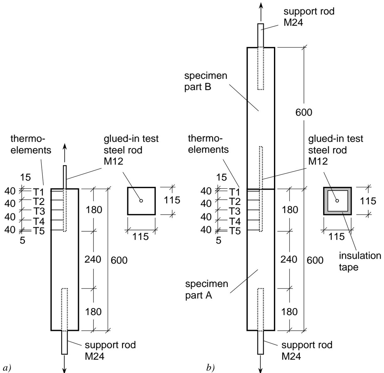
Fig. 1a,b: Geometry and schematic test set-up of
