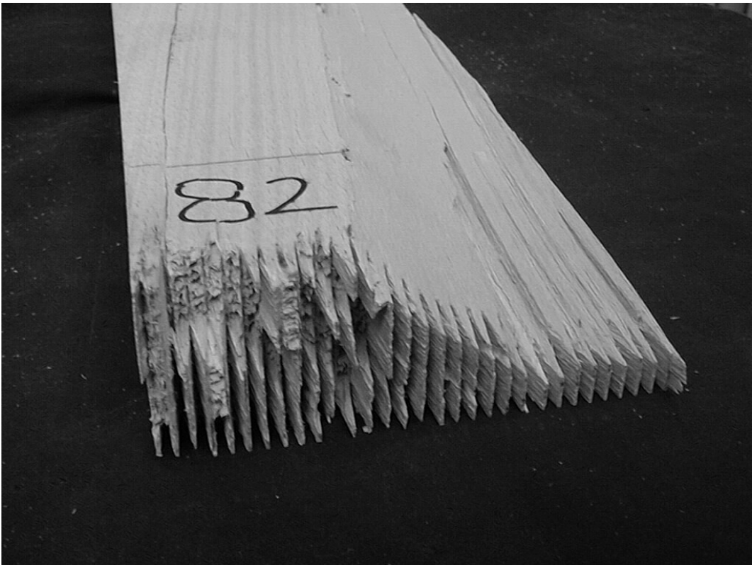
Fig. 4a, b: Views of finger joint tension failures a) "pure" finger joint failure b) "not pure" finger joint failure due to fiber deviation of one adherent with fiber deviation evident from the sloping fracture plane
