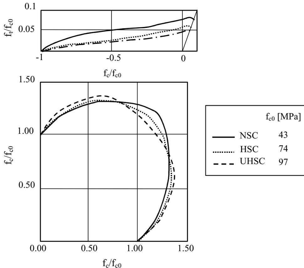
Fig. 2. Biaxial strength envelopes for three types of concrete [Hussein and Marzouk 2000]
