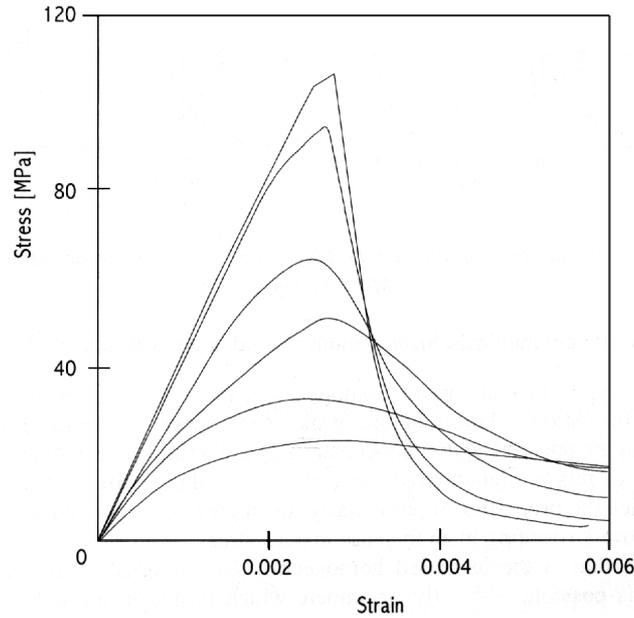
Fig. 3. Stress-strain curves of concrete with various strength grades [Dahl 1992]
