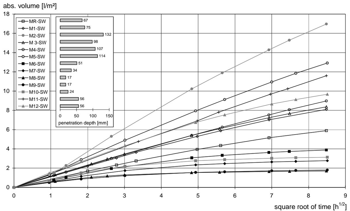
Fig. 4. 72-h-suction tests with water: progression of absorption, penetration depths
