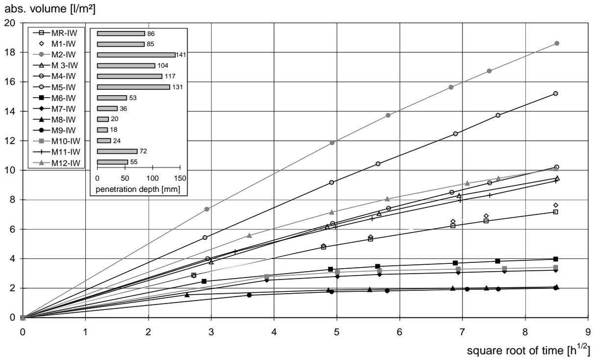
Fig. 5. 72-h-infiltration tests with water: progression of absorption, penetration depths
