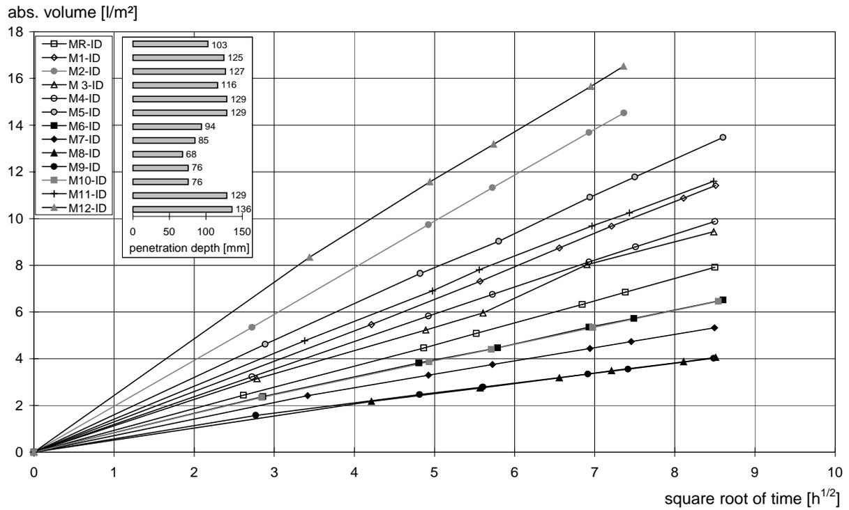
Fig. 3. 72-h-infiltration tests with *n*-decane: progression of absorption, penetration depths
