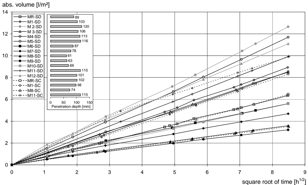
Fig. 2. 72-h-suction tests with n-decane and cyclohexane: progression of absorption, penetration depths
