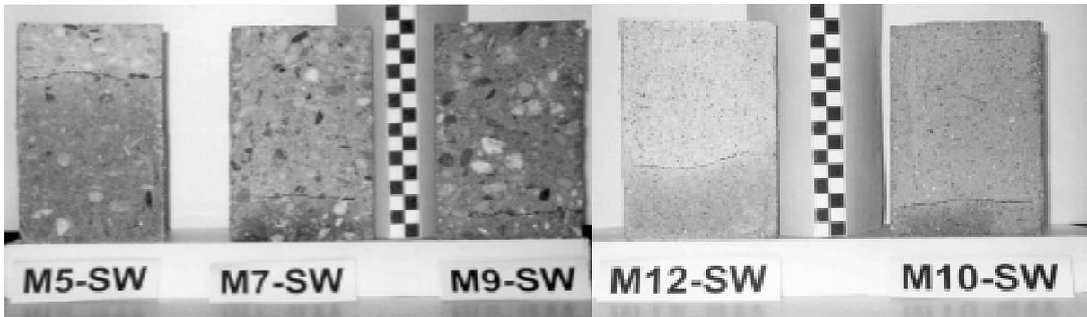
Fig. 6. Splitting surfaces of concretes M5, M7 and M9 and mortars M12 and M10: penetration depths of water after the 72-h-suction test
