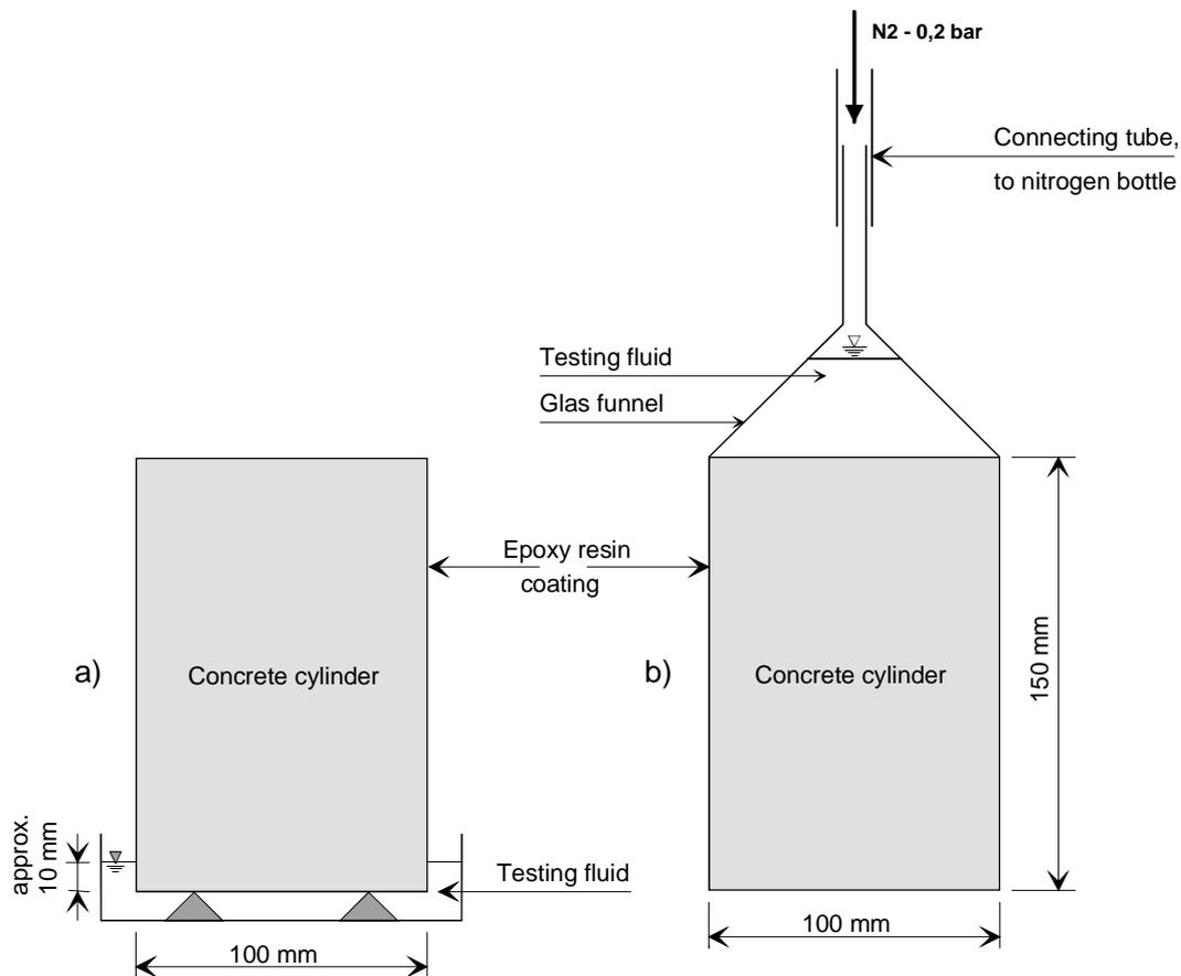
Fig. 1. Experimental setups: a) suction test, b) infiltration test
