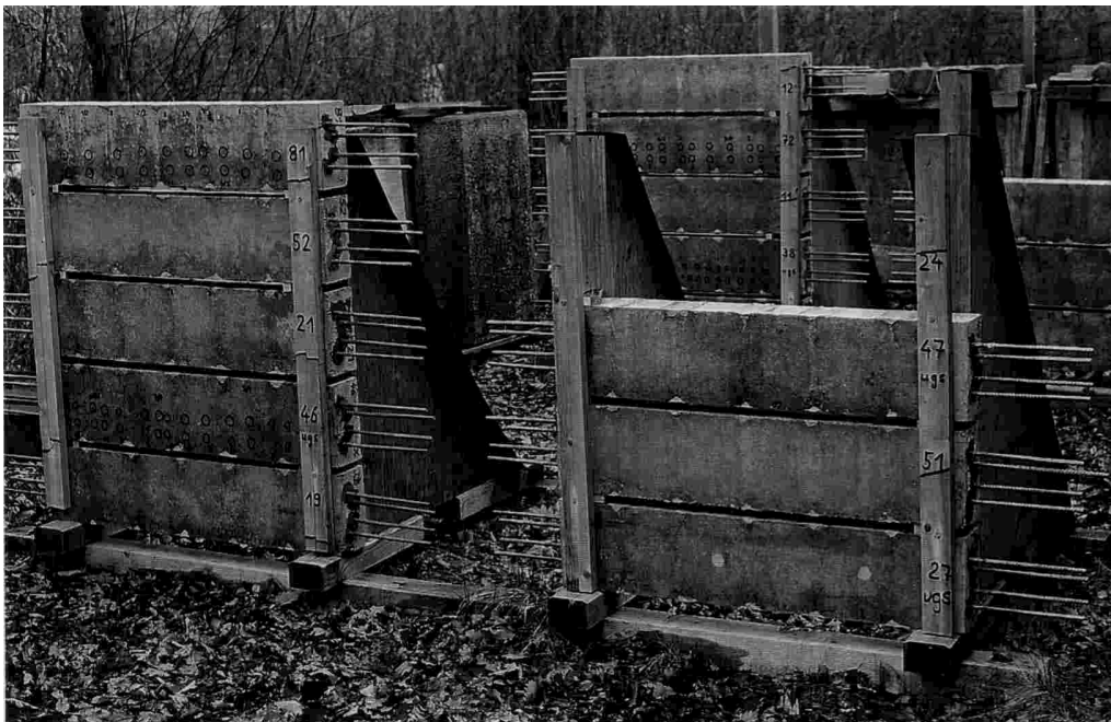
Fig. 7. Storage of cracked concrete specimens under outdoor conditions
